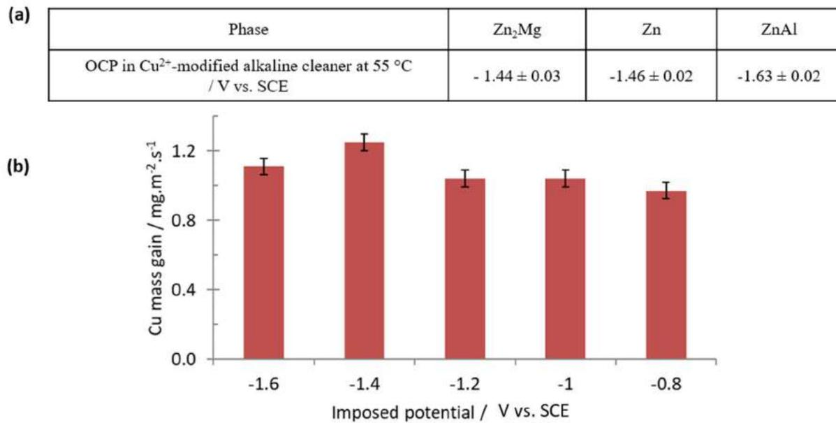
Figure 40: a) Measured OCP of different phases in Cu-modified alkaline cleaner and b) Cu mass gain measured on the Pt electrode as a function of the imposed potential in the Cu-modified alkaline degreasing bath at 55 °C
