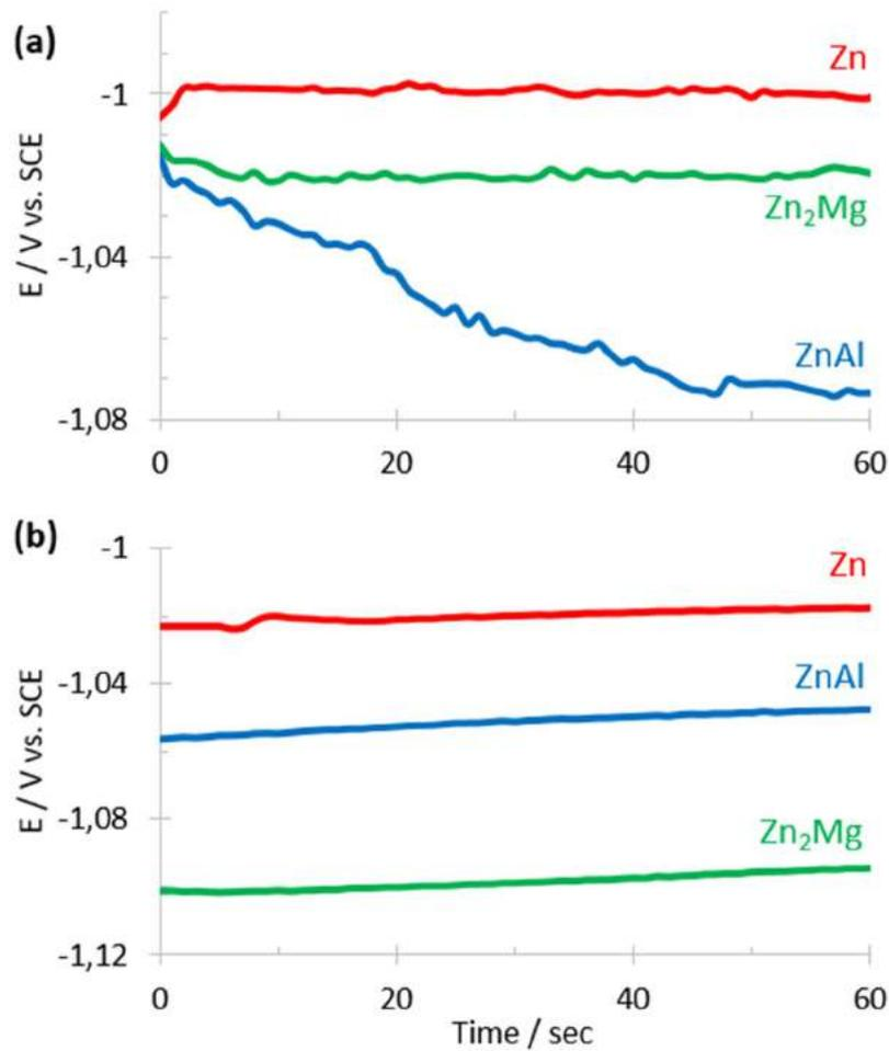
Figure 35: Open Circuit Potentials (OCP) of pure phases in (a) TiCC bath pH 2.6, T=60 °C after 2 min of alkaline degreasing and (b) 5 wt. % Na<sub>2</sub>SO<sub>4</sub> pH 2.6, T=60 °C
