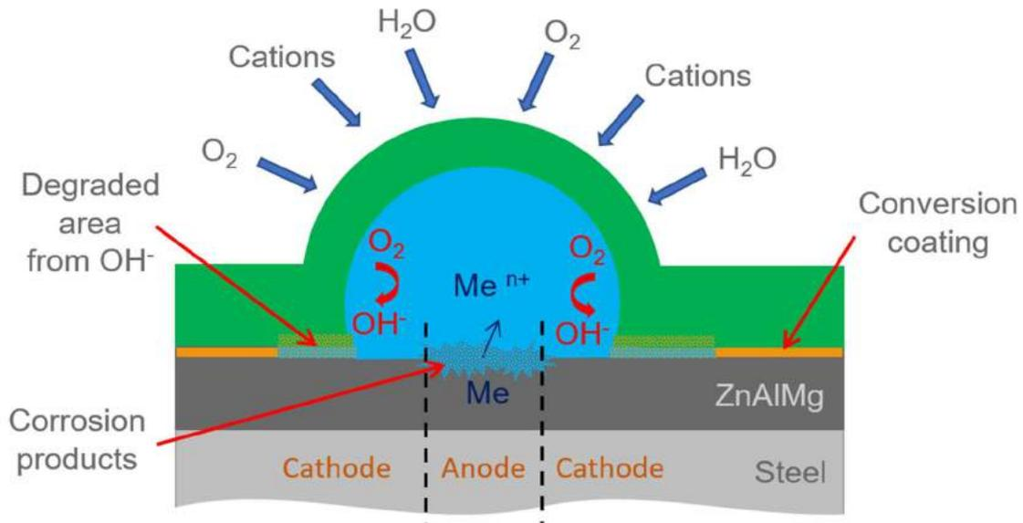
Figure 10: Scheme of the cathodic blistering mechanism
