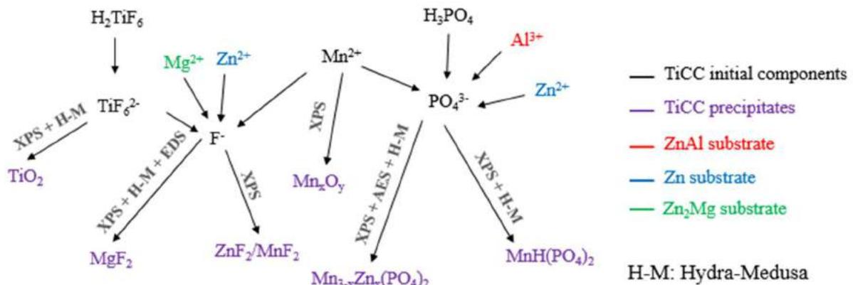
Figure 49: Schematic representation of formation of different CC species during reaction of Zn, ZnAl and Zn<sub>2</sub>Mg phases in TiCC bath
