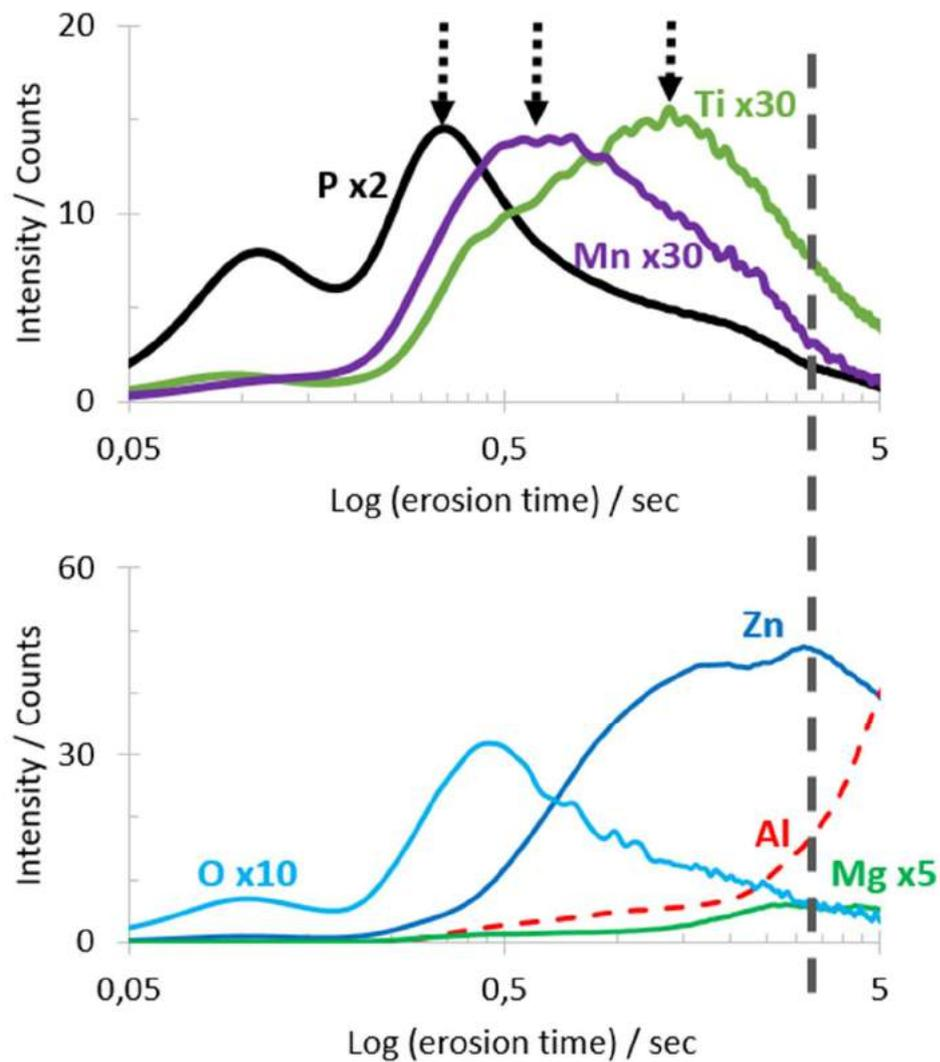
Figure 29: Distribution of P, Ti, Mn and F by GD-OES profile on ZnAlMg after alkaline degreasing followed by immersion in TiCC bath at 60 °C for 30 sec
