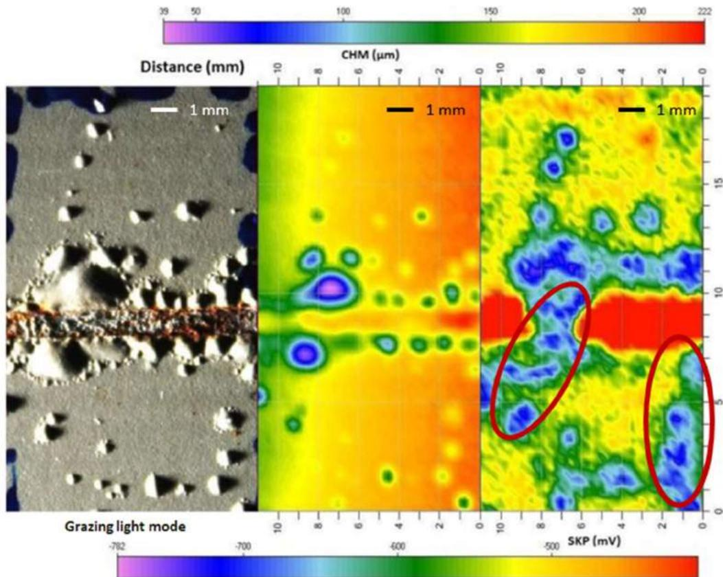
Figure 18: SKP mapping of painted and corroded ZnAlMg material with a down to steel scratch after 24 months of outdoor corrosion testing. The left figure shows optical image, the middle figure shows the topography and the right figure shows the values of Volta potential.
