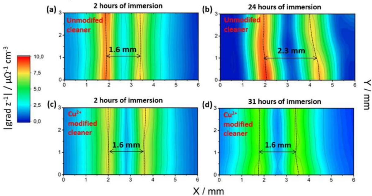
Figure 45: Gradient of the admittance modulus for ZnAlMg degreased with the standard cleaner: (a) after 2 h of immersion, (b) after 24 h of immersion and for ZnAlMg degreased with the  $\text{Cu}^{2+}$  modified cleaner: (c) after 2 h of immersion with alternating, (d) after 31 h of immersion
