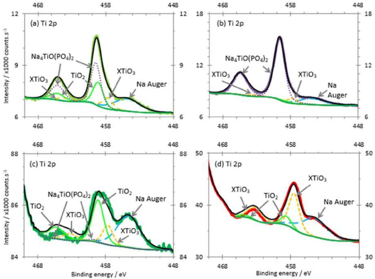
Figure 24: Ti 2p XPS spectra and respective curve-fittings of: (a) as-received activator, (b) dissolved and solvent evaporated activator, (c) Zn<sub>2</sub>Mg and (d) Zn
