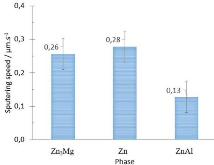
Figure 33: Mean sputtering rates of untreated and polished (4000 SiC) Zn, ZnAl and Zn<sub>2</sub>Mg
