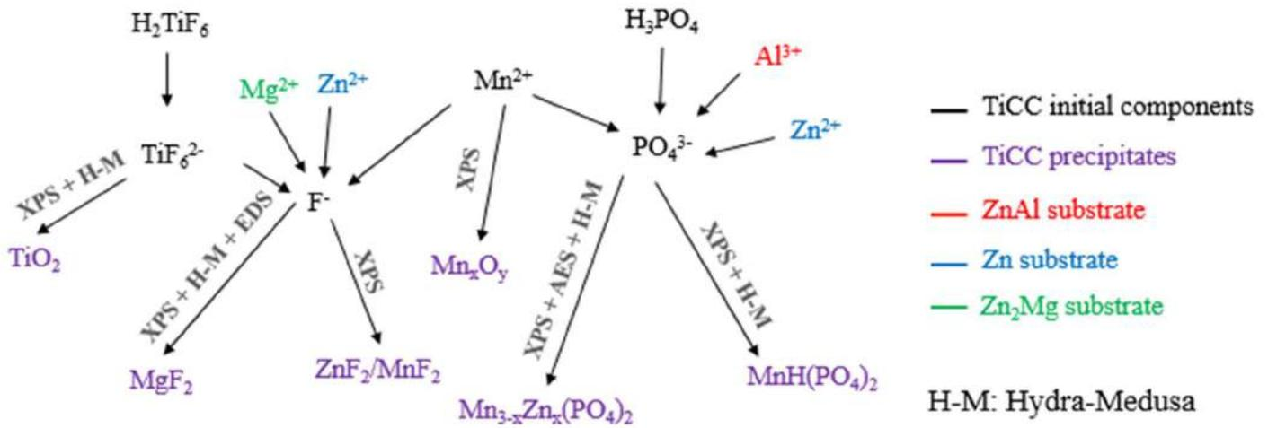
Figure 38: Schematic diagram of the TiCC precipitation on ZnAlMg
