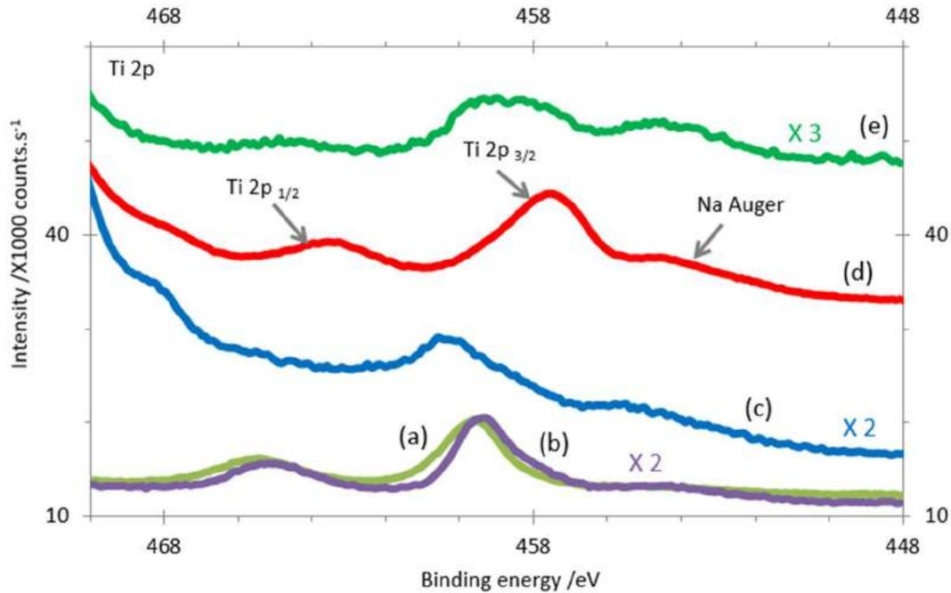
Figure 23: Comparison of Ti 2p XPS spectra of: (a) as-received activator, (b) dissolved and solvent evaporated activator, (c) ZnAl, (d) Zn and (e) Zn<sub>2</sub>Mg
