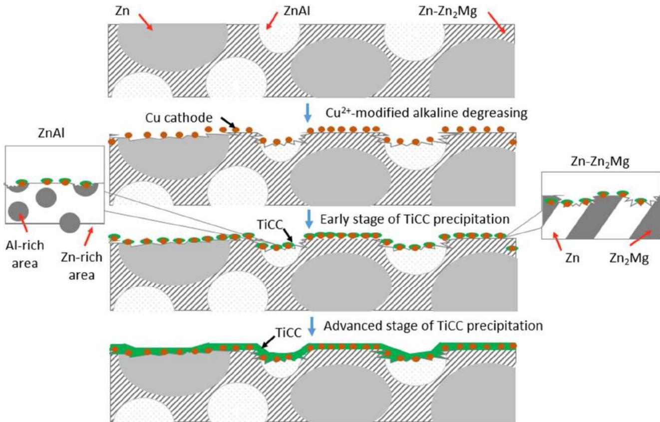
**Figure 52: Scheme of the TiCC precipitation mechanism on ZnAlMg after Cu<sup>2+</sup>-modified alkaline degreasing procedure**
