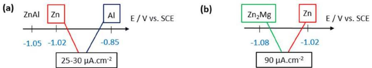
Figure 48: OCP of individual phases and current density measured for galvanic coupling of (a) Zn/Al and (b) Zn/Zn<sub>2</sub>Mg phases relevant for binary eutectics. The measurement was made after 30 min of immersion of uncoupled phases in 5 wt. % Na<sub>2</sub>SO<sub>4</sub> solution with initial pH 2,6 at 25 °C (OCP) followed by 2 h of phase coupling (galvanic current values).
