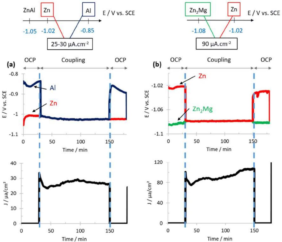
Figure 36: Potential evolution and current density of (a) Zn/Al coupling and (b) Zn/Zn<sub>2</sub>Mg coupling after respectively 30 min of immersion and 2 h of phase coupling in 5 wt. % Na<sub>2</sub>SO<sub>4</sub> pH 2,6 at 25 °C
