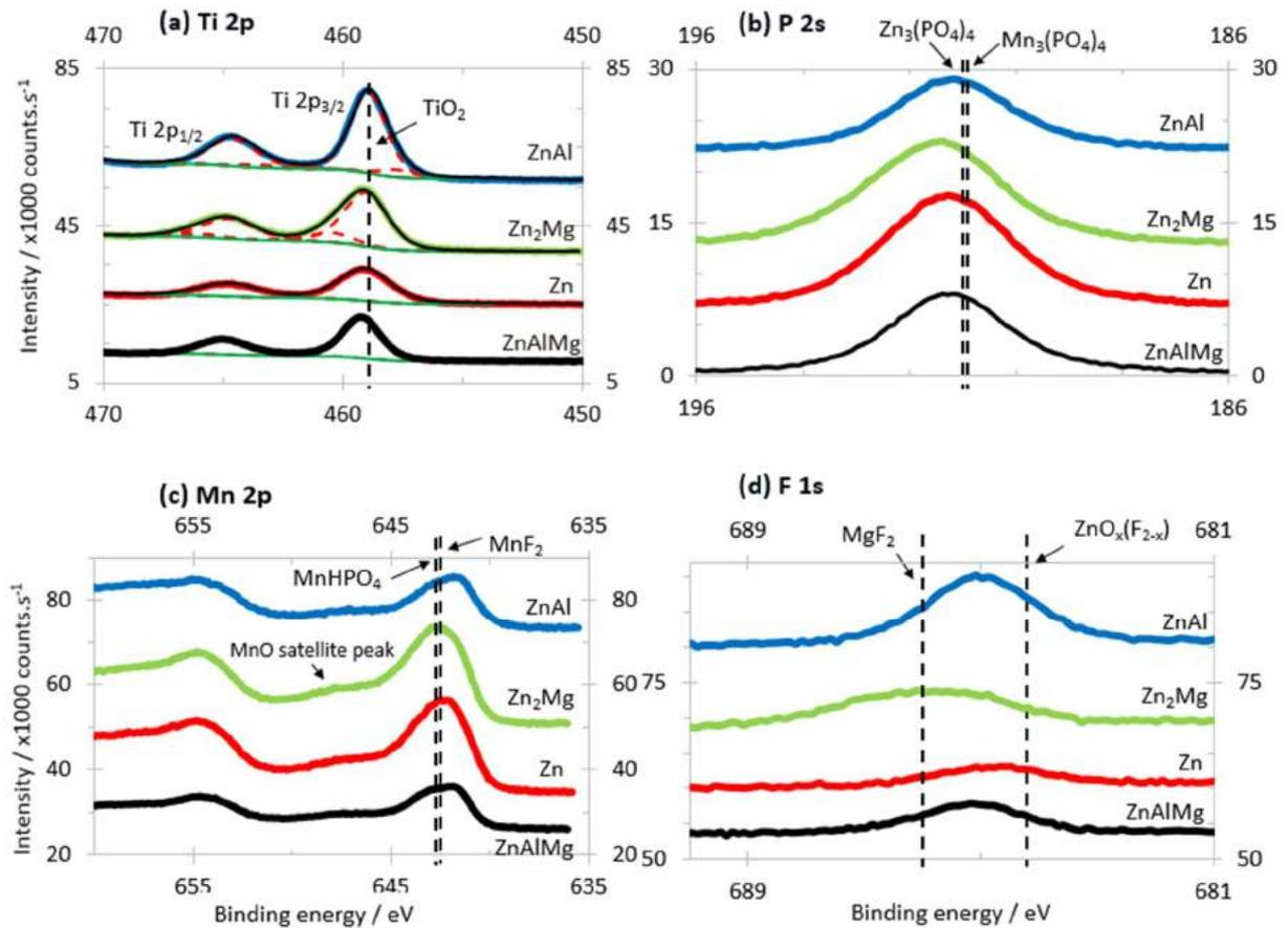
Figure 34: XPS spectra windows of TiCC tracers on pure phases and multiphase ZnAlMg substrates as indicated after standard degreasing and immersion in the TiCC bath at 60 °C for 30 sec
