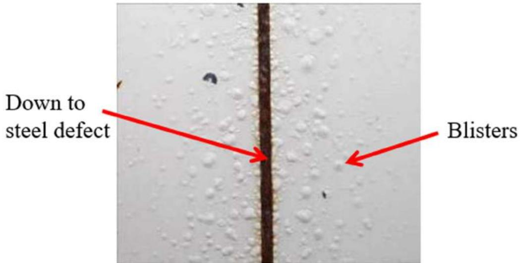
**Figure 7 : Blistering around the down to steel defect after 22 months of natural exposure in a marine environment**
