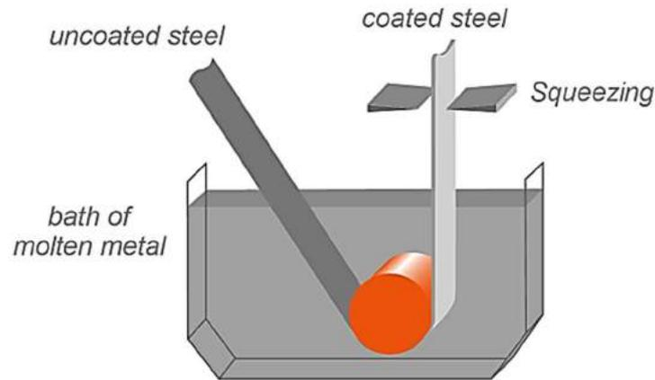
Figure 1: Scheme of the Hot Dip Galvanizing process [10]
