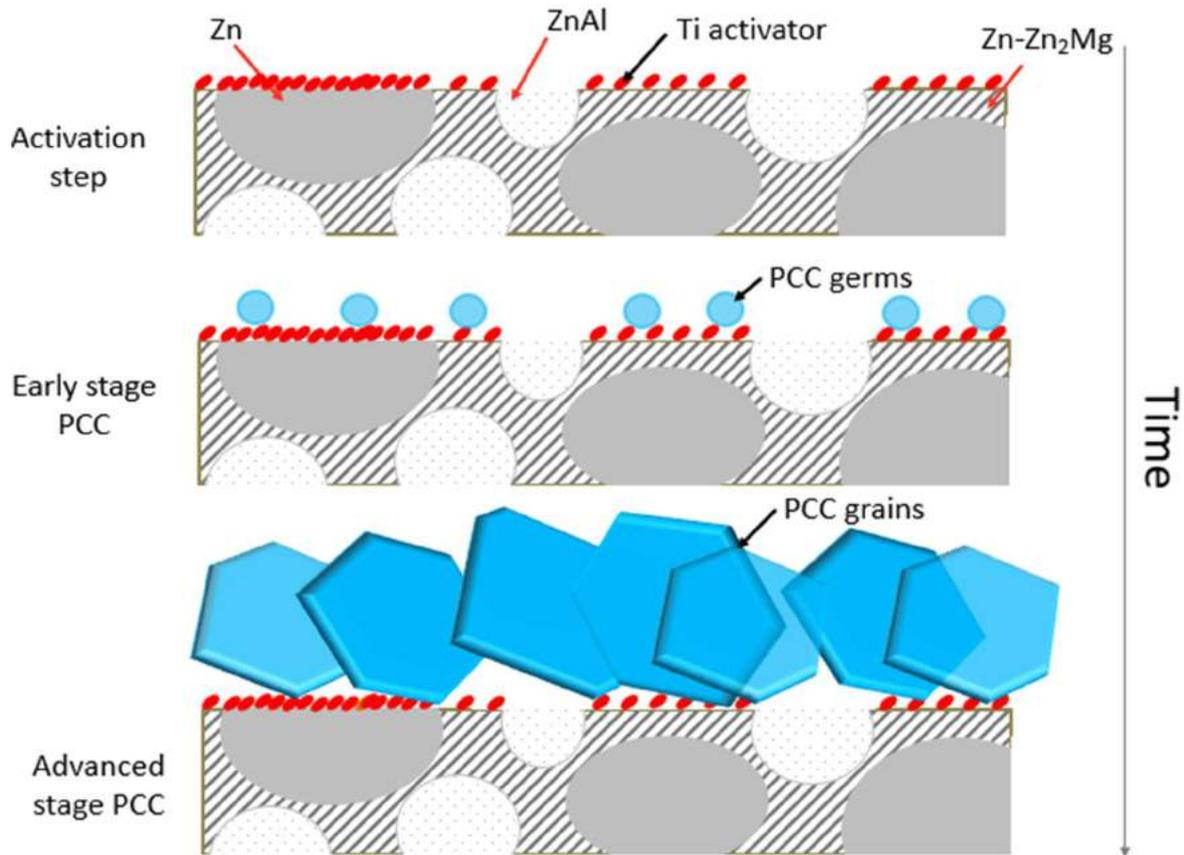
Figure 7: Scheme of the Ti-activator and PCC distributions explaining homogeneous precipitation
