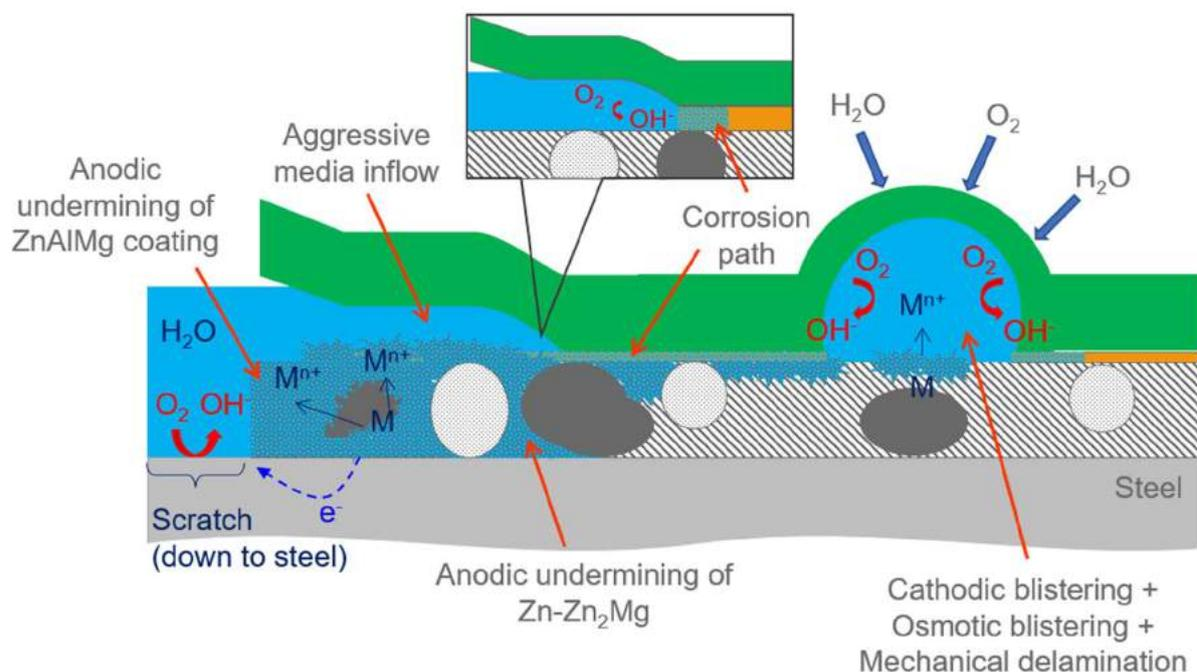
Figure 22: Scheme of the degradation mechanism of painted ZnAlMg material from the down to steel scratch
