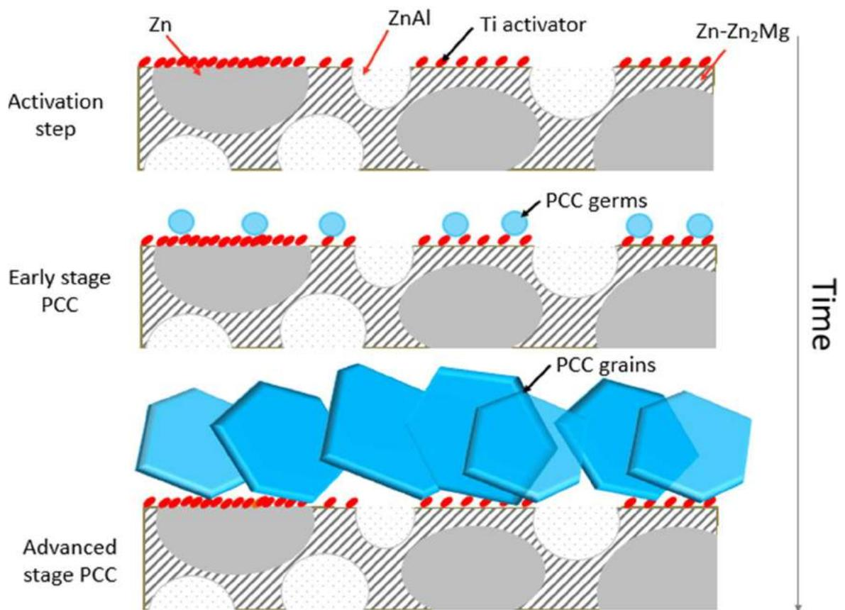
Figure 47: Scheme of the Ti-activator and PCC distributions explaining homogeneous precipitation
