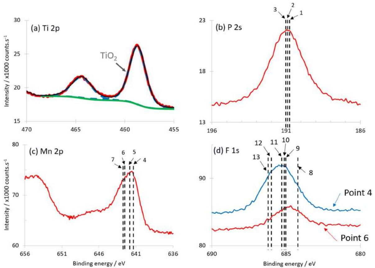
Figure 58: XPS spectra of ZnAlMg after  $\text{Cu}^{2+}$ -modified alkaline degreasing and immersion in the Ti-based CC bath
