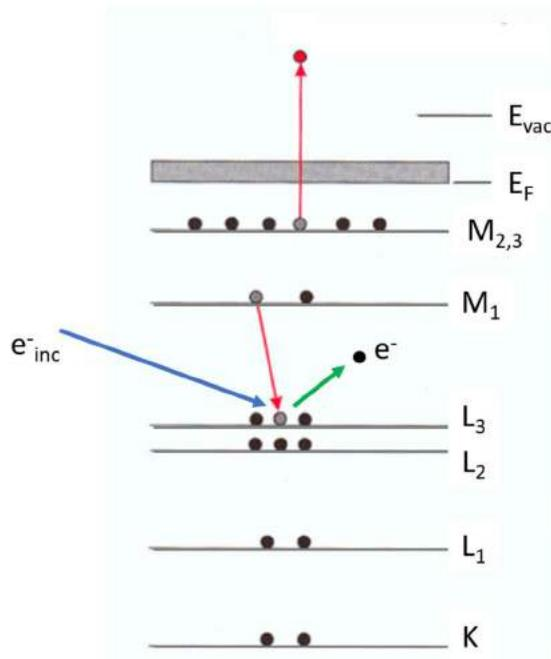
Figure 11: Auger electron emission principle in AES
