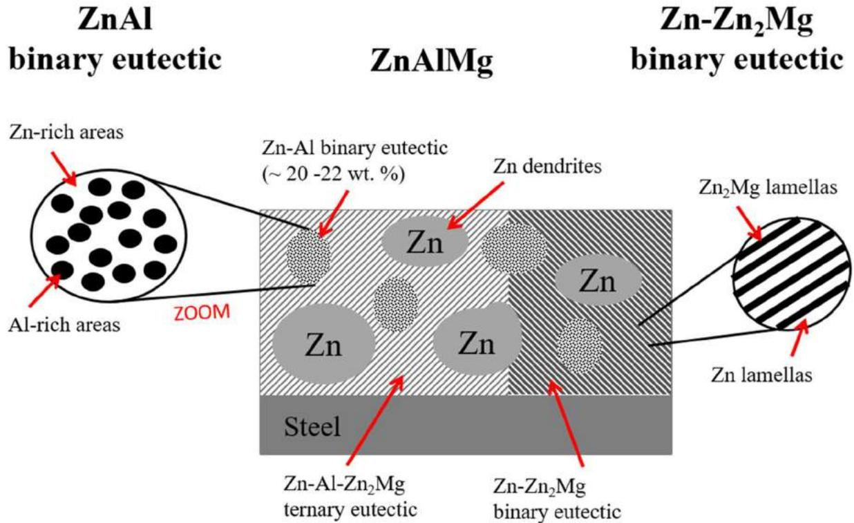
Figure 2: Scheme of the cross-section of ZnAlMg coated steel. Zn-Zn<sub>2</sub>Mg binary phase is composed of bright Zn lamellas and dark Zn<sub>2</sub>Mg ones while the ternary one includes Zn, Zn<sub>2</sub>Mg and an Al mesh. Zn-Al binary phase is composed of bright Zn areas and dark Al-rich ones (inspired by [12])
