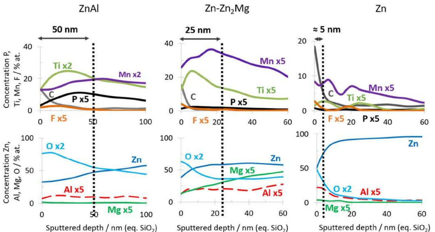
Figure 31: AES profiles of different phases of ZnAlMg after immersion in TiCC bath at 60 °C for 30 sec after standard cleaning
