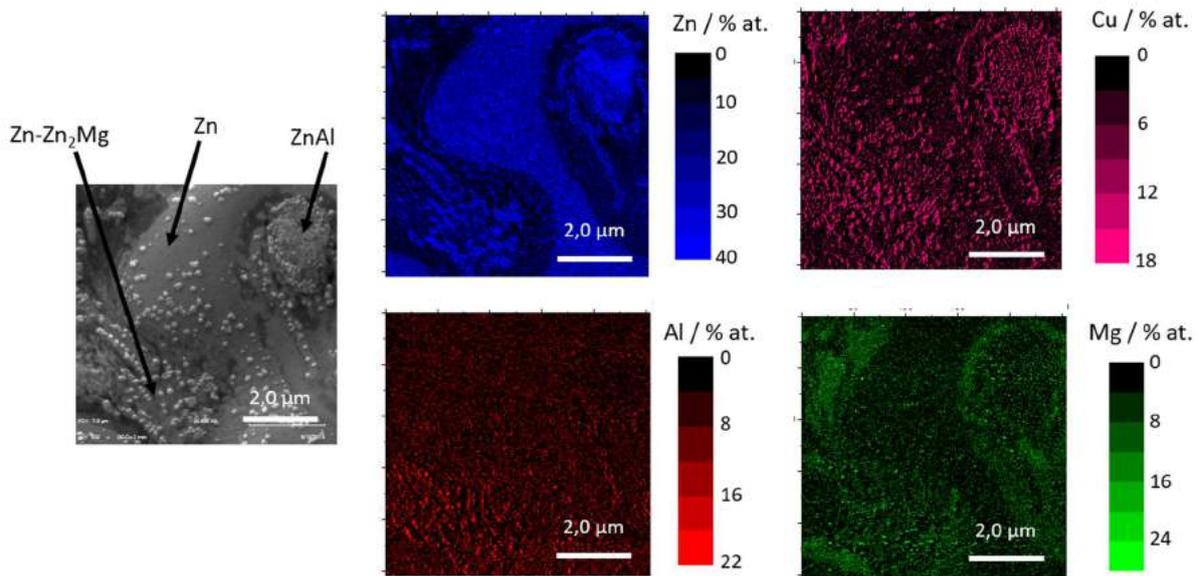
**Figure 51: AES mapping of ZnAlMg surface after immersion in Cu alkaline cleaning at 55 °C for 2 min**
