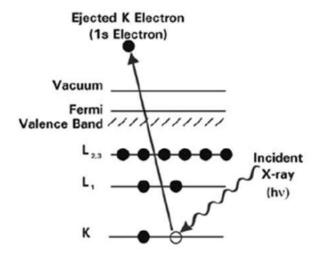
Figure 12: Principle of X-ray photoelectron spectroscopy [7]
