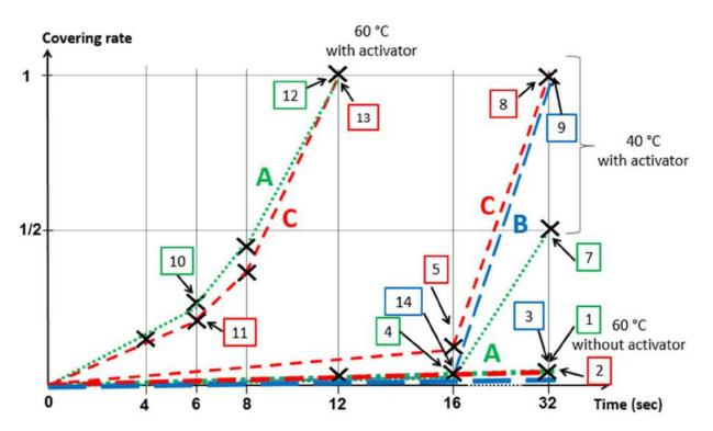
Figure 28: Surface coverage evolution as a function of immersion time, ZnAlMg substrate composition, bath temperature and use of activator (as indicated)
