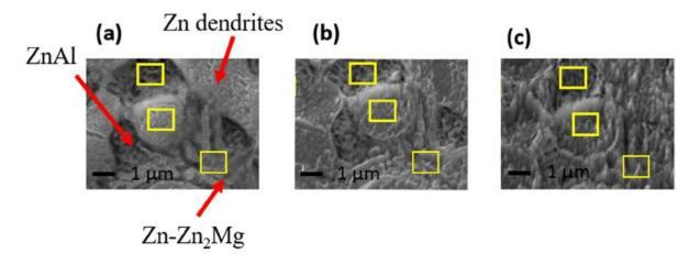
Figure 32: SEM images of ZnAlMg surface after alkaline degreasing and immersion in TiCC bath at 60 °C for 30 sec: (a) before sputtering, (b) after theoretical 70 nm of depth sputtering and (c) after theoretical 300 nm of depth sputtering
