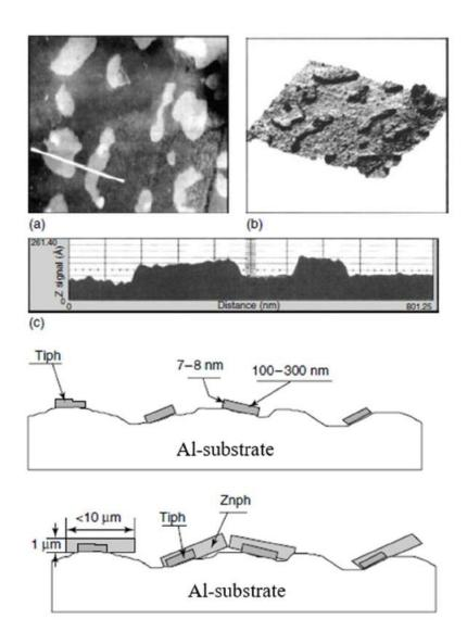
Figure 6: Germination of PCC crystals on sites with adsorbed activator [37]
