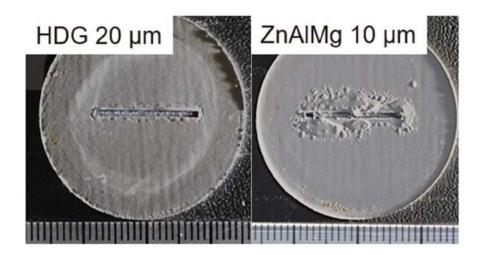
Figure 19: General view of painted HDG and ZnAlMg materials with an artificial defect down to steel after 72 h of anodic galvanostatic polarization in 1 wt. % NaCl solution with initial pH 7.
