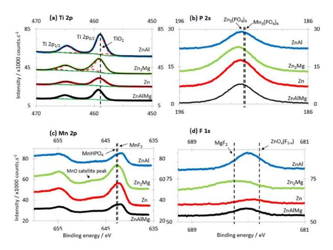
Figure 34: XPS spectra windows of TiCC tracers on pure phases and multiphase ZnAIMg substrates as indicated after standard degreasing and immersion in the TiCC bath at 60 °C for 30 sec
