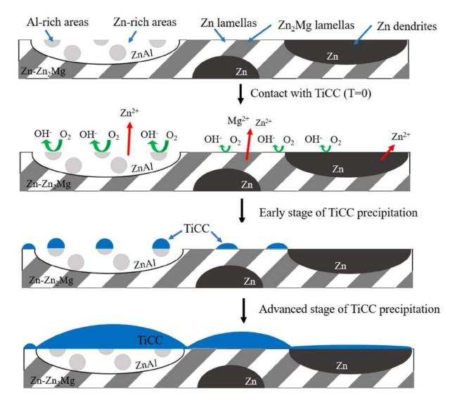
Figure 50: Schematic representation of inhomogeneous TiCC formation on the multiphase substrate
