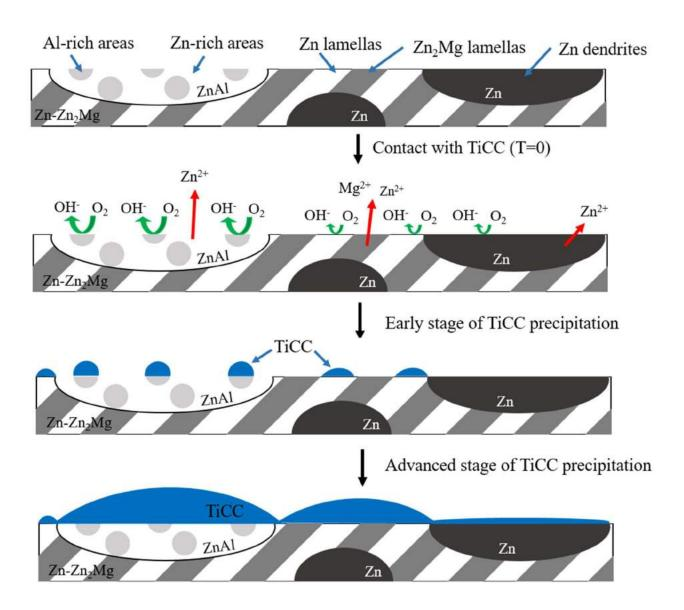
Figure 39: Scheme of the TiCC precipitation mechanism on ZnAlMg
