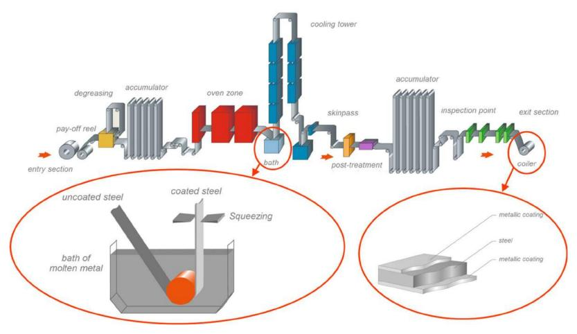
Figure 54: Schematic representation of a hot dip process for ZnAlMg coatings (1]
