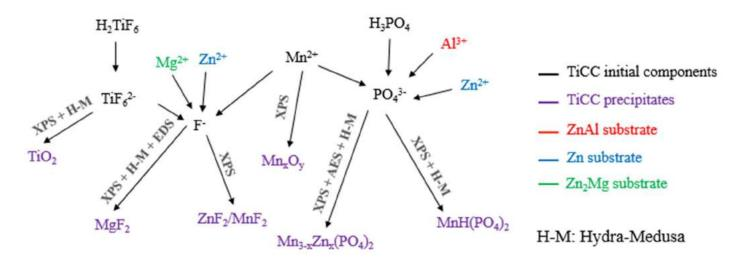
Figure 38: Schematic diagram of the TiCC precipitation on ZnAlMg
