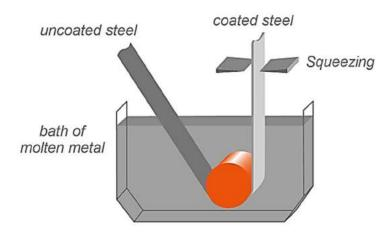
Figure 1: Scheme of the Hot Dip Galvanizing process [10]
