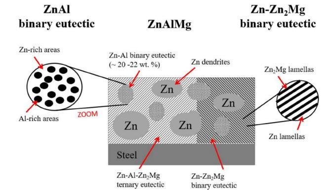
Figure 2: Scheme of the cross-section of ZnAlMg coated steel. Zn-Zn<sub>2</sub>Mg binary phase is composed of bright Zn lamellas and dark Zn<sub>2</sub>Mg ones while the ternary one includes Zn, Zn<sub>2</sub>Mg and an Al mesh. Zn-Al binary phase is composed of bright Zn areas and dark Al-rich ones (inspired by [12])
