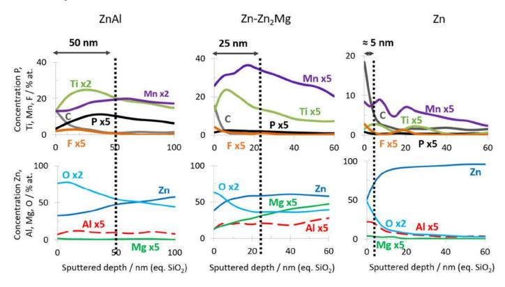
Figure 31: AES profiles of different phases of ZnAlMg after immersion in TiCC bath at 60 °C for 30 sec after standard cleaning
