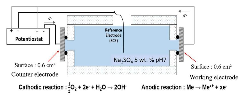
Figure 55: Electrochemical cell used for OCP measurements and galvanic couplings of pure phases (inspired by [2])
