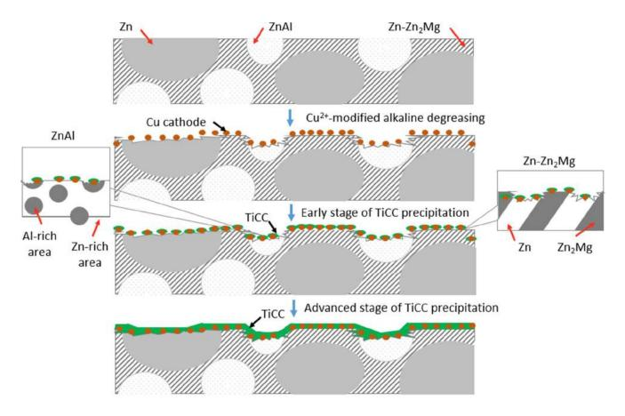
Figure 52: Scheme of the TiCC precipitation mechanism on ZnAlMg after Cu2+-modified alkaline degreasing procedure
