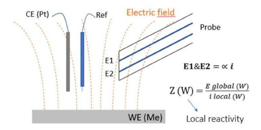
Figure 14: Local Electrochemical Impedance Spectroscopy (LEIS) explanatory diagram
