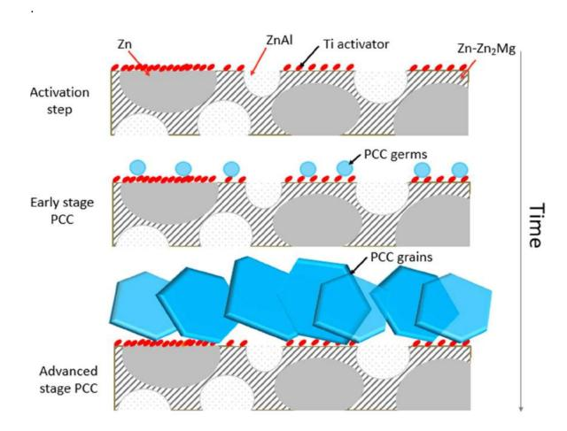
Figure 47: Scheme of the Ti-activator and PCC distributions explaining homogeneous precipitation
