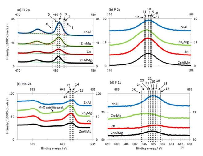
Figure 57: XPS spectra of pure phases and ZnAIMg after standard degreasing and immersion in the TiCC
