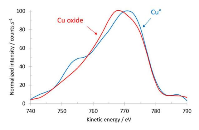
Figure 42: AES deconvolution of Cu auger peak of ZnAlMg after Cu alkaline degreasing for 2 min at 55 °C
