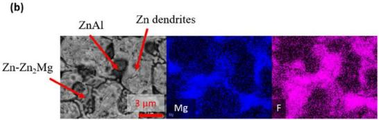
Figure 30: (a) SEM image of ZnAlMg coating (as indicated) after immersion in TiCC at 60 °C for 30 sec and EDS distribution of P, Ti, Mn and F on different phases and (b) SEM image of ZnAlMg and EDS mapping of Mg and F distribution after immersion in TiCC at 60 °C for 30 sec
