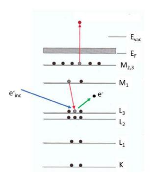
Figure 11: Auger electron emission principle in AES
