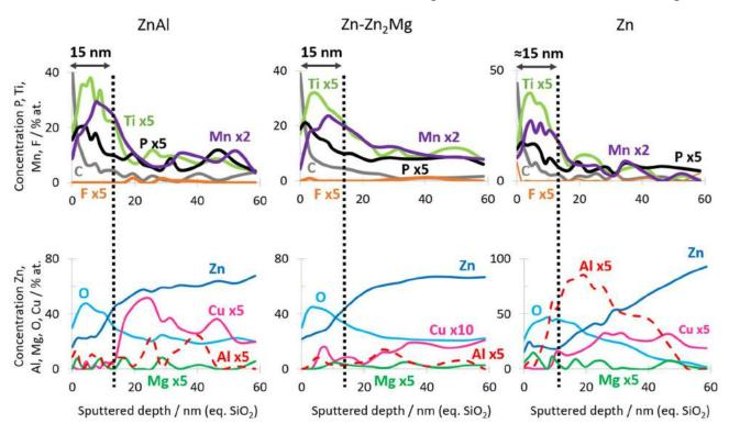
Figure 43: AES profile of ZnAlMg after immersion in TiCC bath at 60 °C for 30sec after Cu alkaline cleaning
