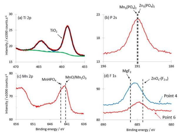
Figure 44: a) Ti 2p, b) P 2s, c) Mn 2p and d) F 1s XPS window spectra of ZnAlMg after Cu<sup>2+</sup>-modified alkaline degreasing and immersion in the TiCC bath at 60 °C for 30 sec
