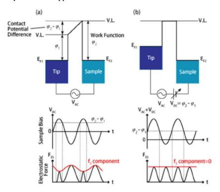
Figure 15:Scheme of the SKP principle
