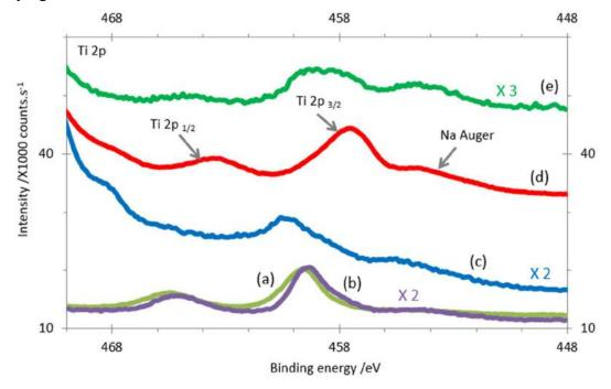
Figure 23: Comparison of Ti 2p XPS spectra of: (a) as-received activator, (b) dissolved and solvent evaporated activator, (c) ZnAI, (d) Zn and (e) Zn<sub>2</sub>Mg
