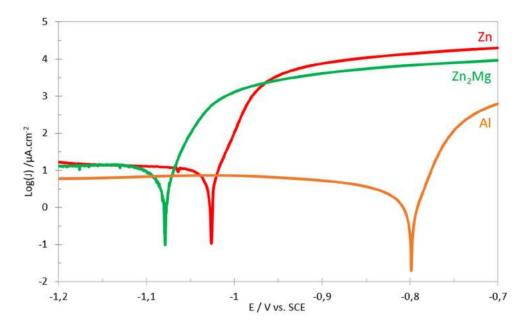
Figure 21: Anodic and cathodic polarization curves of pure phases relevant for ZnAlMg coating in 5 wt. %
