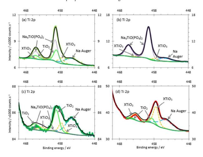
Figure 24: Ti 2p XPS spectra and respective curve-fittings of: (a) as-received activator, (b) dissolved and solvent evaporated activator, (c) Zn2Mg and (d) Zn
