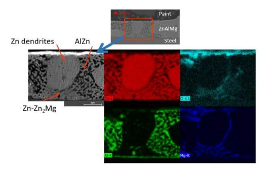
Figure 20: SEM-EDS mapping of ZnAlMg material after 72 h of anodic galvanostatic polarization in 1 wt. %
