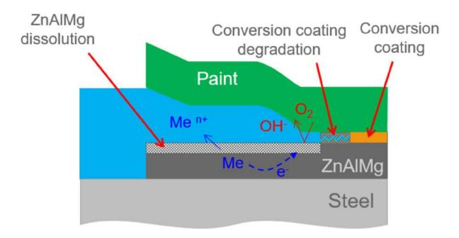
Figure 9: Cathodic delamination mechanism
