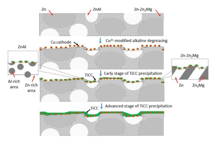
Figure 46: Scheme of the TiCC precipitation mechanism on ZnAlMg after Cu2+-modified alkaline degreasing procedure
