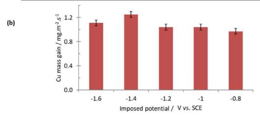
Figure 40: a) Measured OCP of different phases in Cu-modified alkaline cleaner and b) Cu mass gain measured on the Pt electrode as a function of the imposed potential in the Cu-modified alkaline degreasing bath at 55 °C
