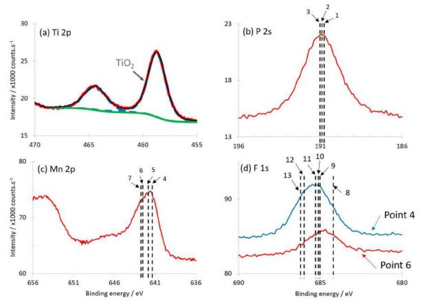
Figure 58: XPS spectra of ZnAlMg after Cu2+-modified alkaline degreasing and immersion in the Ti-based CC
