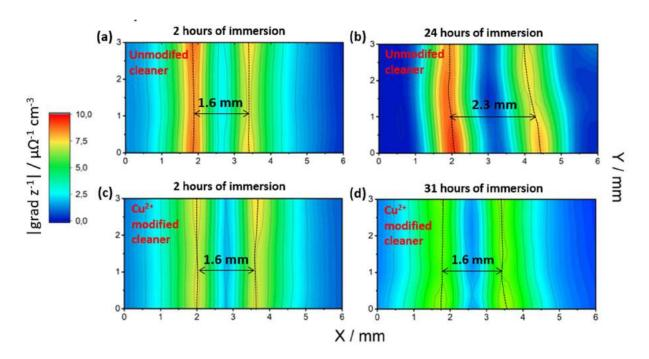
Figure 45: Gradient of the admittance modulus for ZnAlMg degreased with the standard cleaner: (a) after 2 h of immersion, (b) after 24 h of immersion and for ZnAlMg degreased with the Cu<sup>2+</sup> modified cleaner: (c) after 2 h of immersion with alternating, (d) after 31 h of immersion
