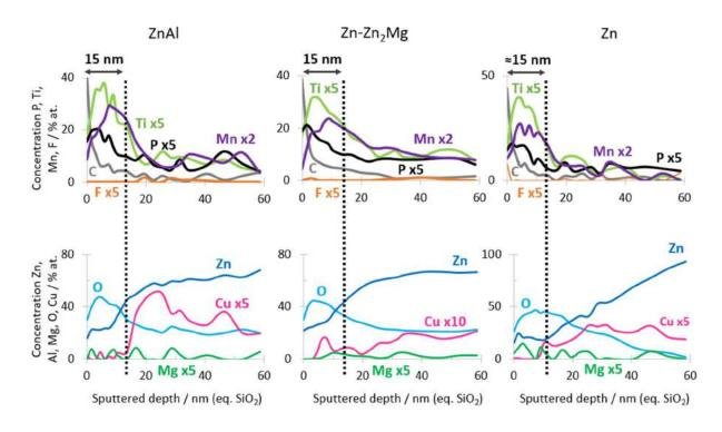
Figure 53: AES profile of ZnAlMg after immersion in TiCC bath at 60 °C for 30 sec after Cu alkaline cleaning
