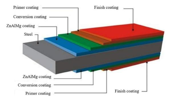
Figure 3: Structure of a painted ZnAlMg coated steel for the pre-painted market
