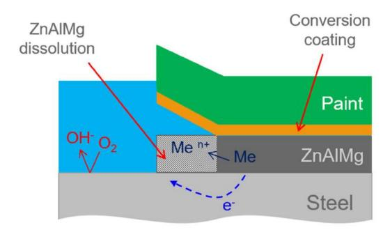
Figure 8: Anodic delamination mechanism
