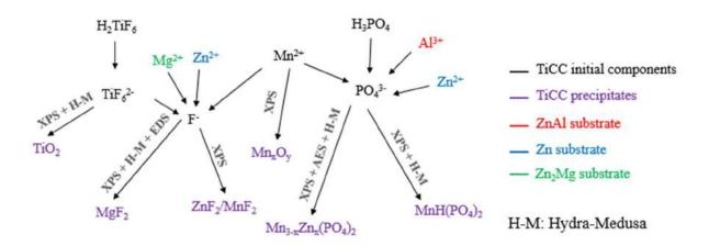
Figure 49: Schematic representation of formation of different CC species during reaction of Zn, ZnAl and Zn2Mg phases in TiCC bath
