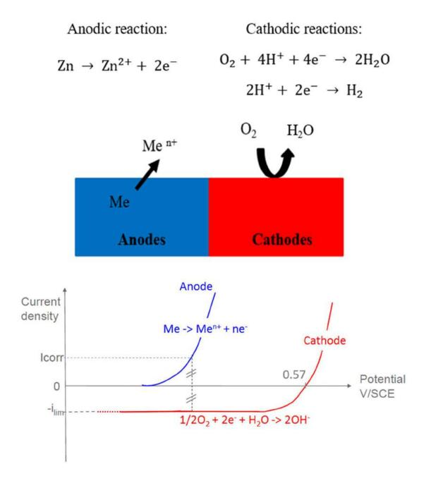
Figure 4: Schematic representation of anodic and cathodic reactions distribution during galvanic coupling
