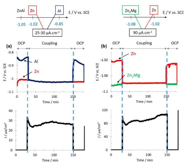
Figure 36: Potential evolution and current density of (a) Zn/Al coupling and (b) Zn/Zn2Mg coupling after respectively 30 min of immersion and 2 h of phase coupling in 5 wt. % Na2SO4 pH 2,6 at 25 °C
