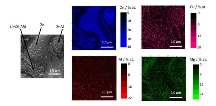
Figure 41: AES mapping of ZnAlMg surface after immersion in Cu alkaline cleaning at 55 °C for 2 min
