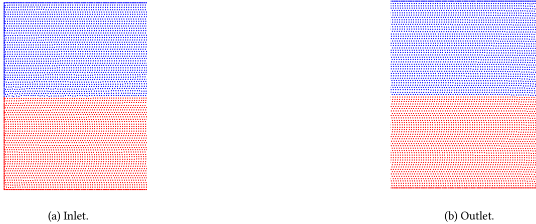
Figure 3.31: Two-phase separated Poiseuille flow with open boundaries: focus on the volume fraction field at inlet and outlet at t = 2800 s for a density ratio of 100.
