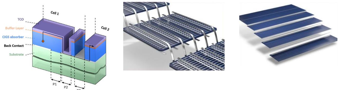
Figure 1.13 – Illustration showing different methods of cell integration in a module [38]. **Left** – Monolithic integration. **Center** – Stringing and Tabbing method. **Right** - Shingling method.
