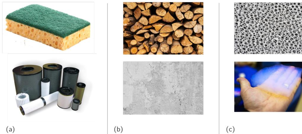
Figure 1.1: Examples of common porous media. (a) Industrial products: washing sponge and fuel filters. (b) Building materials: wood logs and concrete wall. (c) Engineered materials: low-density ceramic foam and aerogel.
