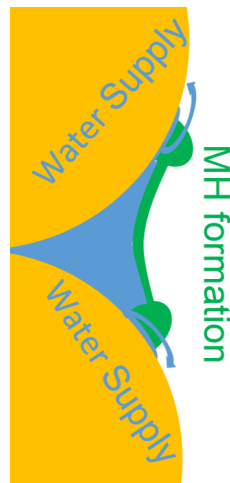
Figure 7.3: Schematic of the first mechanism of MH formation under gas-excess conditions.
