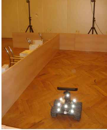
Figure 4.3: Wifibot robot in its testing arena, surrounded by Optitrack cameras
