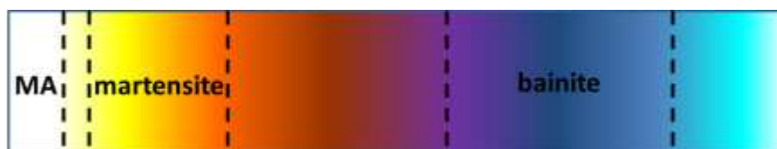
Figure 114: Full range of coloration that has been encountered using LePera etching on carbide free upper bainite for the present study.
