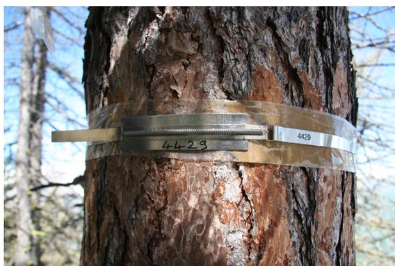
Figure 2.15: Manual band dendrometer on a tree stem
