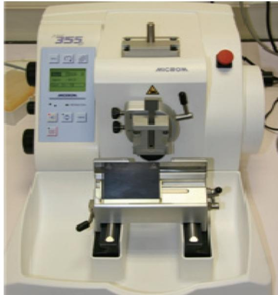
Figure 2.22: Rotary microtom, (Photo by M.Harore).
