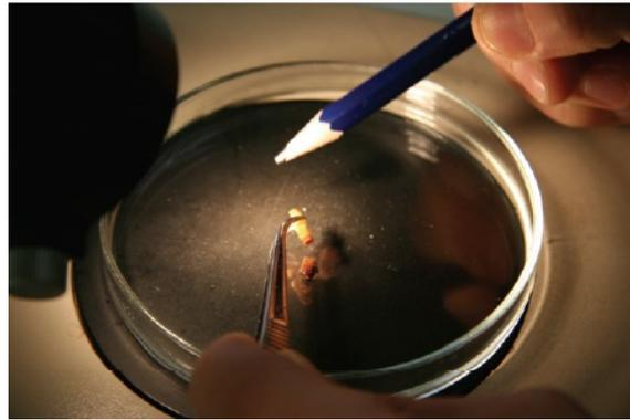
Figure 2.19: Marking the upper face of microcore using a pencil, (Photo by M.Harore).
