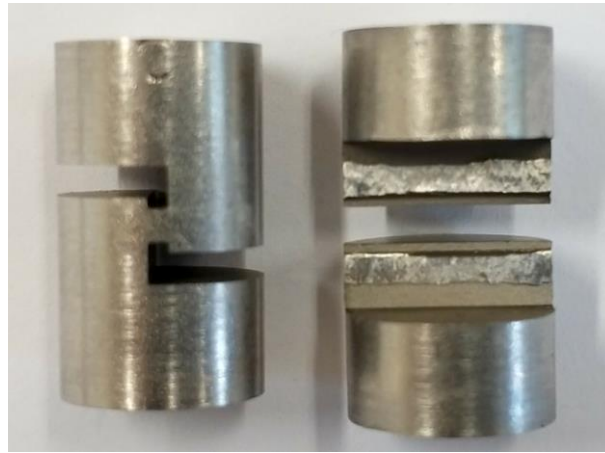
Fig. 3.6. The SSS specimens before and after tests at a nominal shear strain rate of 6000 \text{ s}^{-1} .
