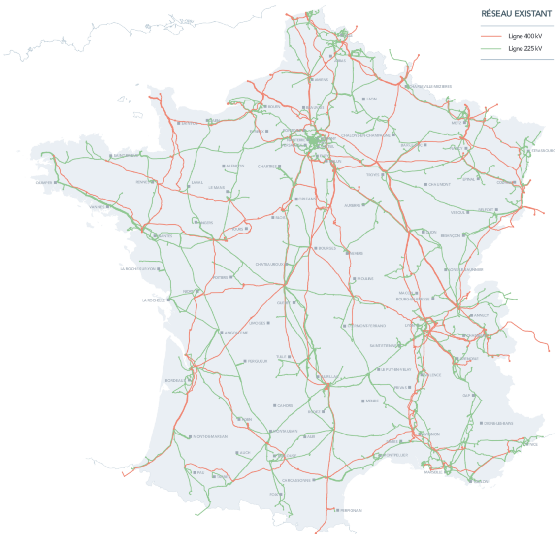
FIGURE 1.3: The French high-voltage network [RTE, 2019b].
