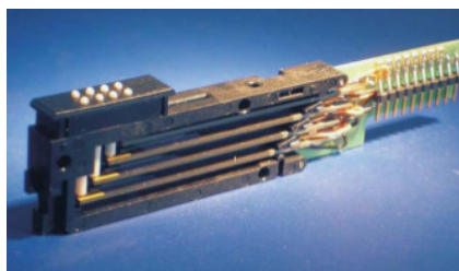
(b) A piezoelectrically actuated Braille cell.
