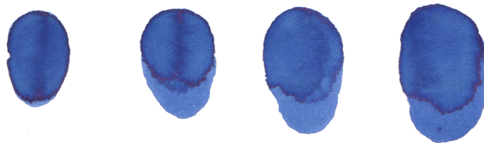
Figure B.1: Inked surface of paper as a function of applied force (from left to right, 0.2 N, 1.5 N, 3.0 N and 7.0 N).
