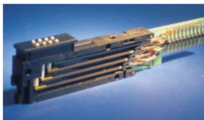
(b) A piezoelectrically actuated Braille cell.
