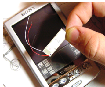
Figure 2.12: The TouchEngine, a 0.5 mm thick piezoelectric bender actuator, from [67].
