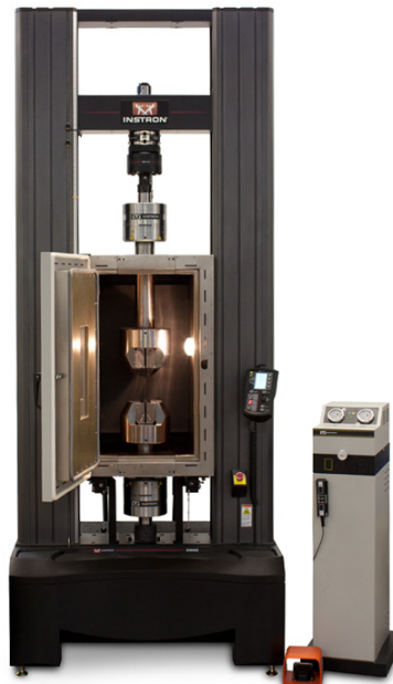
FIGURE 2.12: Tensile tests setup: Instron machine ref 5980
