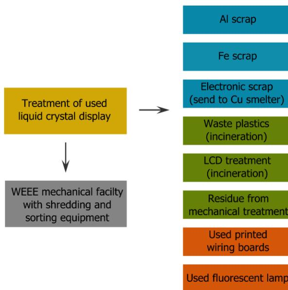
Figure 5-2. Ecoinvent modulation for treatment of used LCD displays.
