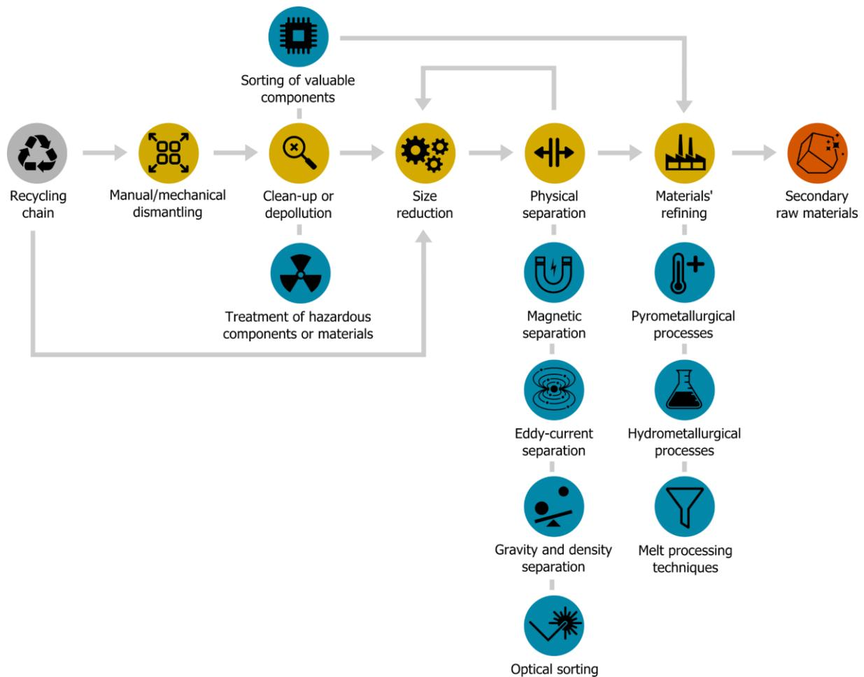
Figure 4-7. Schematic flowsheet of recovery of secondary raw materials from e-waste.
