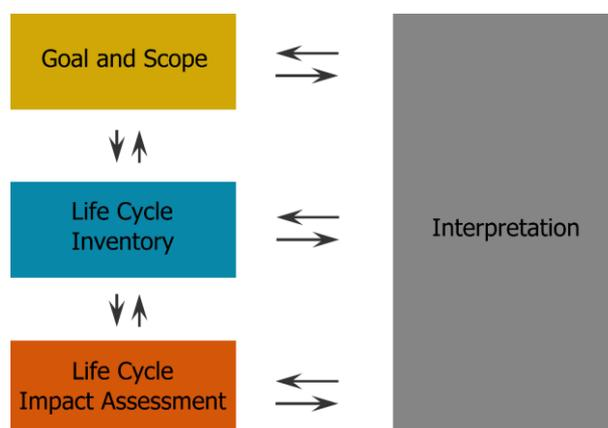
Figure 5-1. LCA phases according to ISO (2006a).
