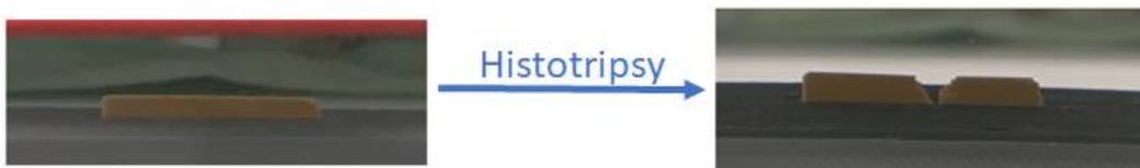
Figure 66 - Result of the alignment verification protocol when both transducers are aligned
