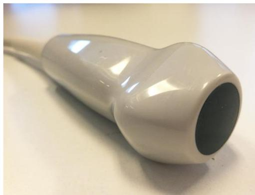
Figure 48 - PAXY probe including a convex cylindrical acoustic lens
