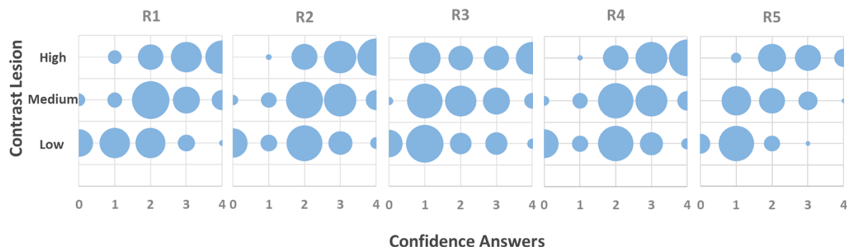
Figure 6.14: Confidence levels for each iodine concentration (High= 0.8\text{mg}/\text{cm}^3 , Medium= 0.5\text{mg}/\text{cm}^3 , Low= 0.3\text{mg}/\text{cm}^3 ). Confidence level 0 is attributed to missed lesions. The size of the disks is proportional to the percentage of answers given by the reader for a specific iodine concentration and a specific confidence level.
