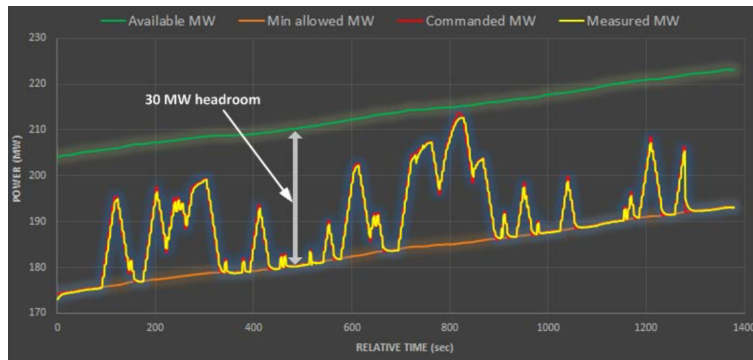
Figure 1.5: Provision of aFRR by a PV power plant of 300 MW capacity, illustration by NREL [5]
