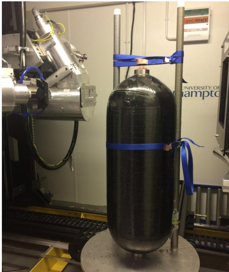
Figure 4.1: The carbon-epoxy pressure vessel inside a tomograph.
