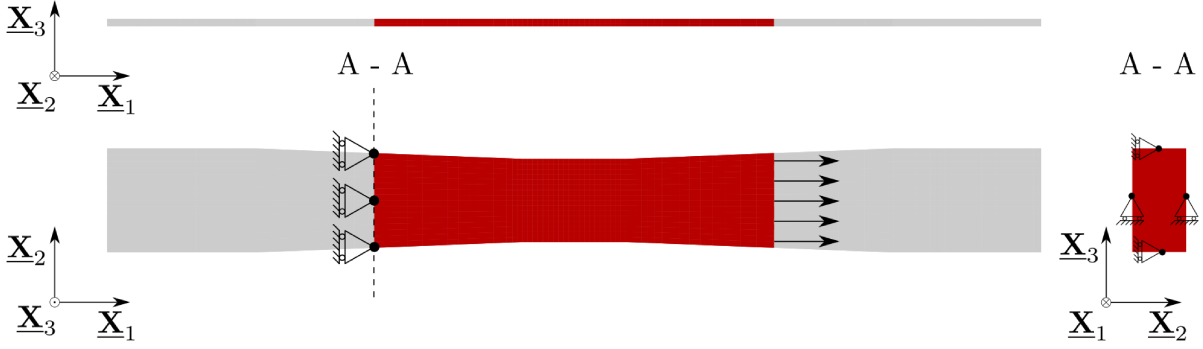
Figure 3.6 Sketch of the tensile specimen geometry with the simulated part marked in red.
