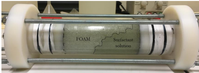
Fig. 2.6 In situ foam generation in foam generator column (after 0.6 PV injection):
