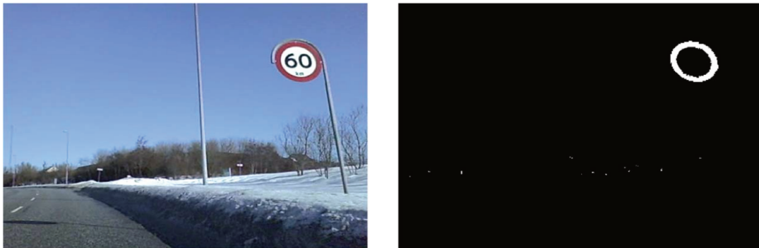
Figure 3.4: Segmentation of red color in HSI space [Møgelmoose et al., 2012]
