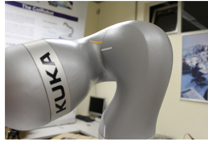
Figure 4.8: Joint four near the limit, yellow and white markers are nearing each others.
