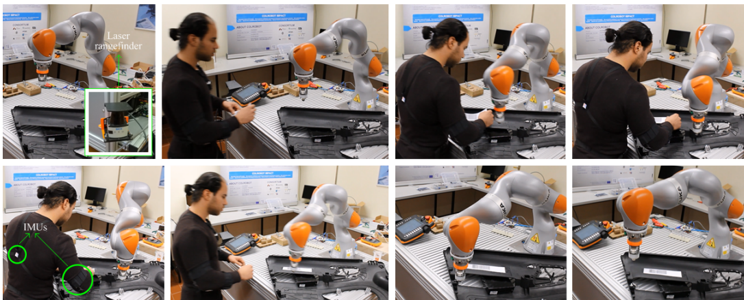
Figure 3.21: Test 3. Collaborative robotic cell for car door card assembly (video segment showing the experiment is in [6]).
