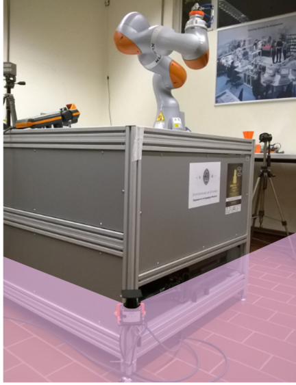
Figure 3.9: Laser scanner mounted at the level of the coworker’s legs in the base of the table holding the robot. If the robotic arm is installed on a mobile platform the solution is similar.
