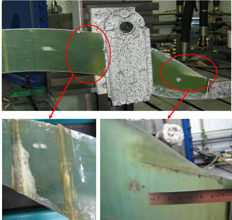
FIGURE 3.31 – Zone de rupture de la lame composite de configuration 2
