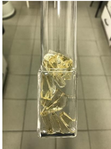
Figure 4.2: Glass samples placed in a silica crucible just before being place in the in-situ observation apparatus.
