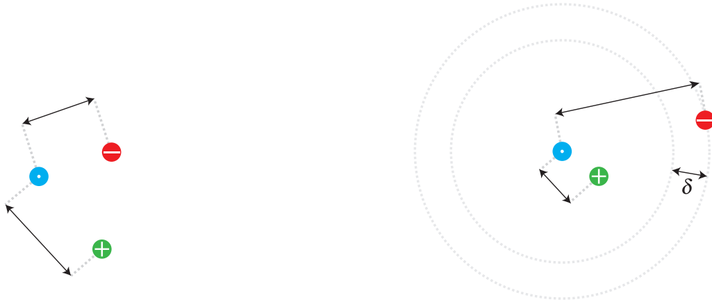
(c) With triplet loss, the representation of the positive pose is closer to the representation of the anchor pose than the negative one. The negative one is at least at a distance \delta of the anchor one.
