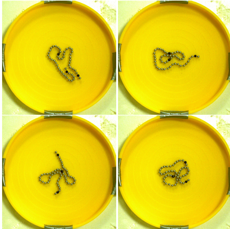
Figure 8.13 – Snapshots of a vibrated 50 monomers long granular chain taken at different times. The black beads are the ones tracked during the experiment.
