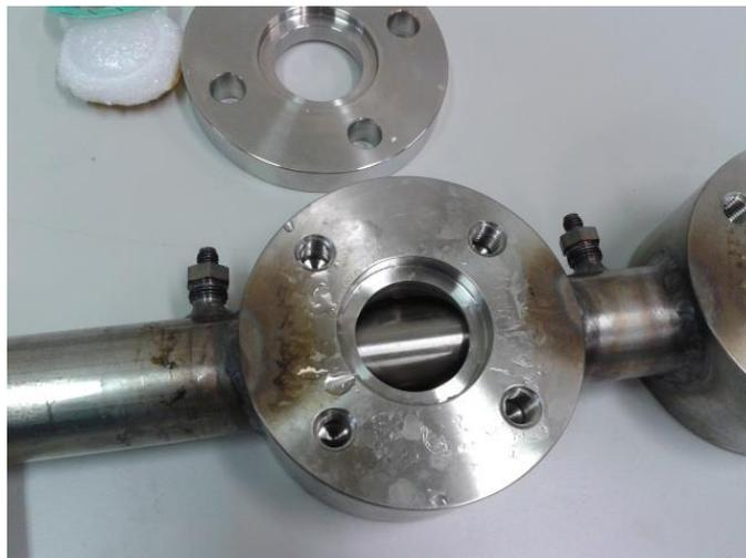
Figure 102: Observation windows of the CO<sub>2</sub> condensation phenomenon (HB01, HB02, HB03, HB04).
