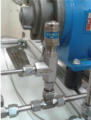
Figure 99: Safety valve for NOVEC 7100 non-flammable refrigerant (SP02).
