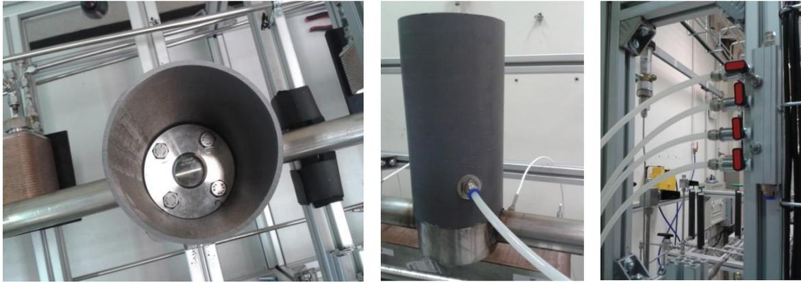
Figure 103: Portholes, seals and inerting / dehumidifying system
