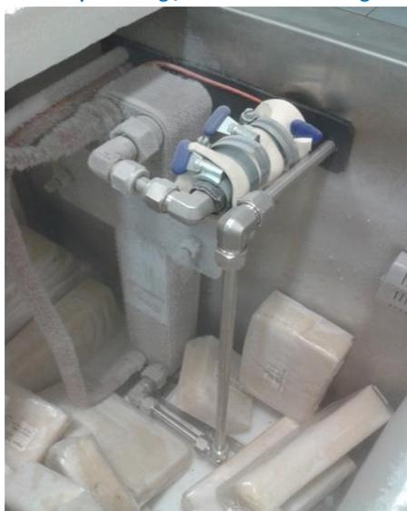
Figure 98: Cooling system (ECO1), minimum temperature of  $-164^{\circ}\text{C}$  (LABOLOGIC Model LA - ZW128)
