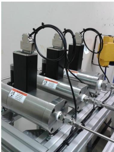
Figure 101: Brooks flow meters for each gas with inerting zone (FC01, FC02)
