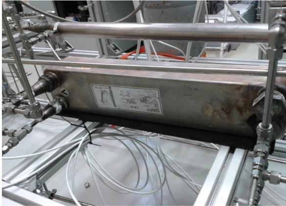
Figure 105: Heat recovery exchanger (ECO2).
