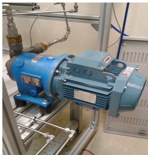
Figure 97: Refrigerant pump Brand AB (PP01) for flow rates up to 250 g / s NOVEC 7100 refrigerant
