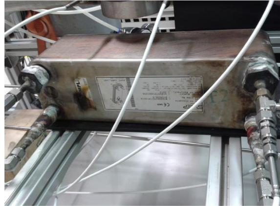
Figure 106: Heat exchanger (ECO3).
