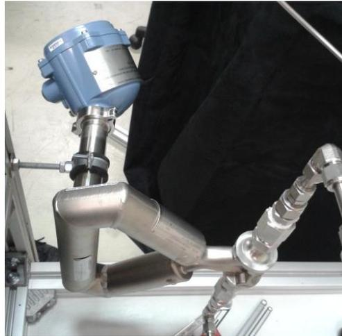
Figure 100: Emerson Coriolis refrigerant flowmeter -200 ° C
