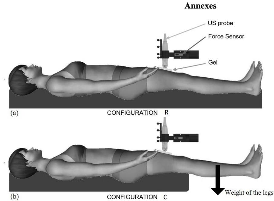
*Figure 1: 1a. Configuration R, the subject is in a relax state and compressions are applied on the anterior mid-thigh. The experimental setup composed of the US probe and the force sensor is described in this figure. 1b. Configuration C, the legs of the subject are not lying on the bed, so that anterior muscles of the thigh are contracted.*
