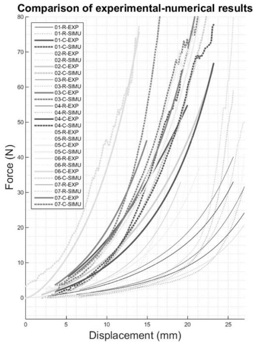
Figure 4: Comparison of experimental and numerical force-displacement curves for all subjects with one operator in both configurations. Thin lines represent configuration R, wide lines represent configuration C. Experimental curves are represented in continuous lines and numerical curves in dotted lines.
