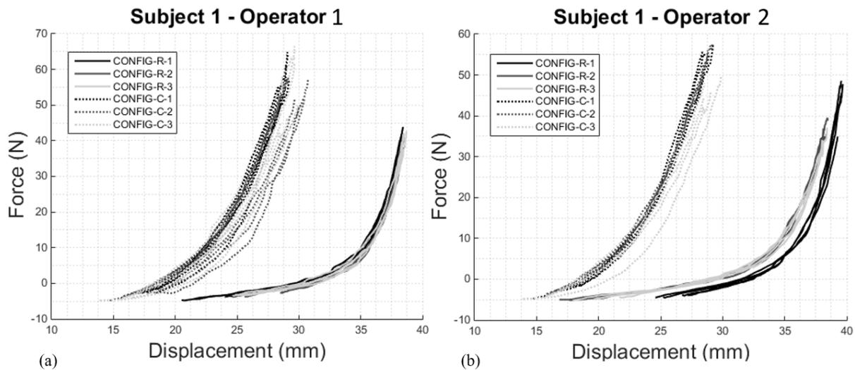
Figure 3: 3a. Experimental force-displacement curves obtained by operator 1 for one subject. The two colours correspond to the two cycles of indentation. 3b. Experimental force-displacement curves obtained by operator 2 for one subject. The two colours correspond to the two cycles of indentation.
