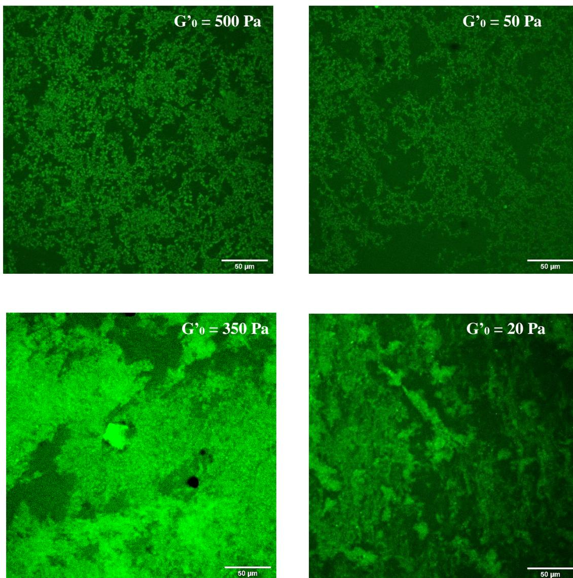
*Figure V.5: Images of peanut protein gels ( $C_p = 12\text{g}/100\text{g}$ ) obtained by CSLM (magnification  $\times 40$ ). Proteins are stained in green. Gelation was obtained by Thermal Treatment (TT, top), or by an enzymatic pre-treatment before the thermal treatment (eTT, bottom). Proteins were extracted and gelled at 0.5M (left) or 0.8M (right). Scale bar are 50  $\mu\text{m}$ .*
