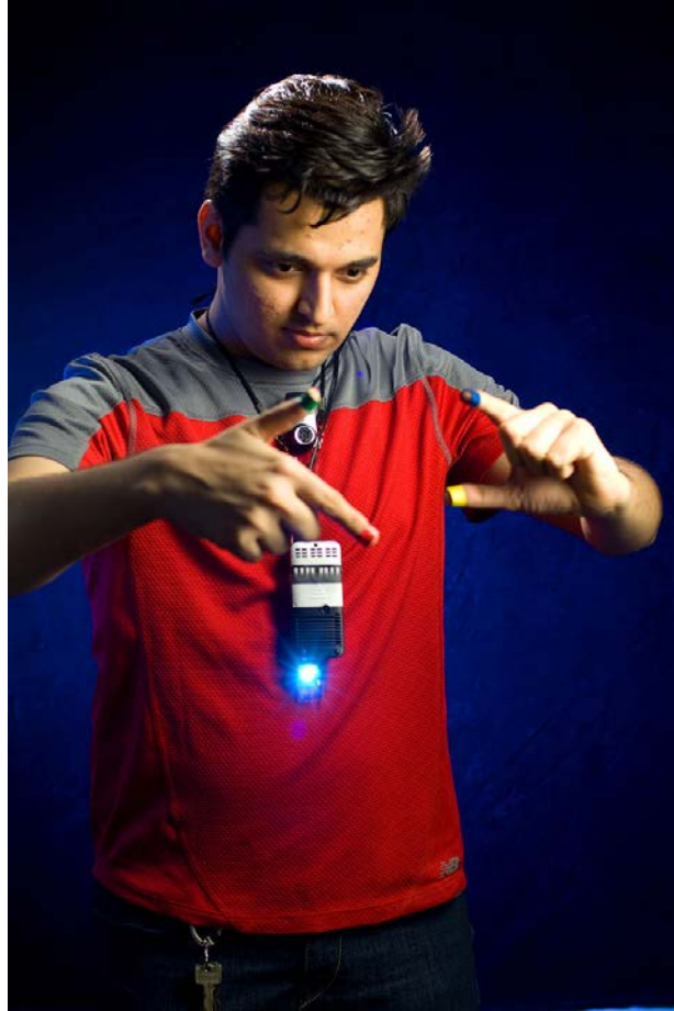
Fig. 24. Pranav Mistry's gestural interface, as part of the "Wear your World" (WUW) suite places affordances at the center of software and hardware design. A projector and a camera track hand gestures and interpret them, while projecting contents on any surface, including one's own hand.
