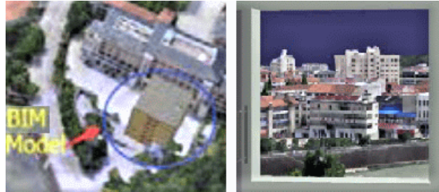
Figure 2.14: Juxtaposition of photogrammetry and 3D BIM model in a MR application for building sales, from two points of view - Sun et al. courtesy [163]
