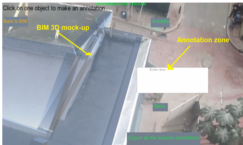
Figure 3.4: Construction supervision: a user adding annotation to signal a difference between as-built and as-planned models in our MR prototype
