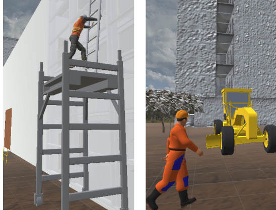
Figure B.1: Two examples of hazardous situations in a virtual worksite: on the left, an example of a fall hazardous situation, on the right a struck-by hazardous situation
