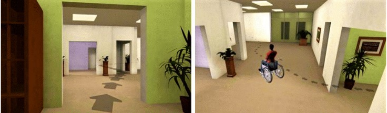
Figure 2.12: BIM-Game engine prototype for collaborative design, using two different points of views, first-person on the left and third-person on the right - Yan et al. courtesy [187]
