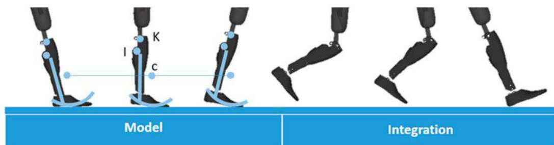
Figure 33: Knee joint center (K) trajectory estimation from a shank mounted MIMU (positioned at I) using the roll over shape paradigm (C representing the center of the foot roll-over-shape). Taken from (Duraffourg et al. , 2019)
