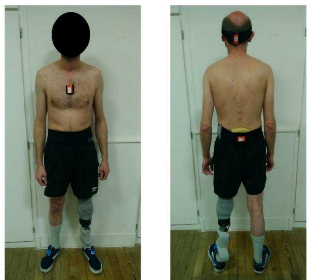
Figure 48: Participant equipment with IMUs and insoles. For the acquisitions, IMUs on the pelvis, sternum, and head were positioned under the Velcro straps to prevent sensors sliding.
