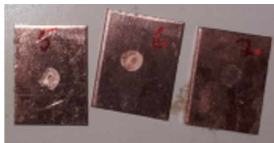
Figure D.8: Picture of the front surface of 3 samples after laser shock. In this case the diameter of shock was 4 mm. The circular spots in the center of the copper sample correspond to the impacts of the laser. Picture by Michel BOUSTIE.
