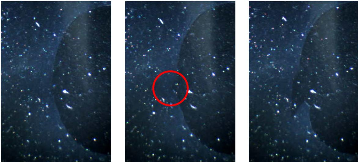
Figure 3.32: Propagation and deviation of a fracture at  $\lambda \approx 2.5$  in a pure-shear sample of  $\text{Ni}^{2+}$  dual-crosslink hydrogel.
