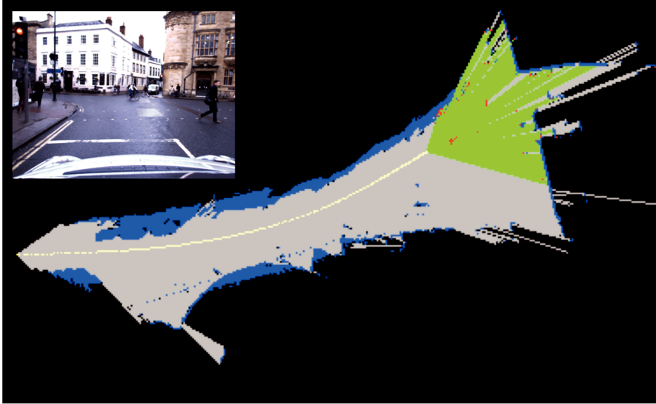
Figure 4.9: Global map after performing temporal fusion. The colors represent the different states of the life-long grid: CF (green), CU (gray), CO (red), FO (blue) and U (black).
