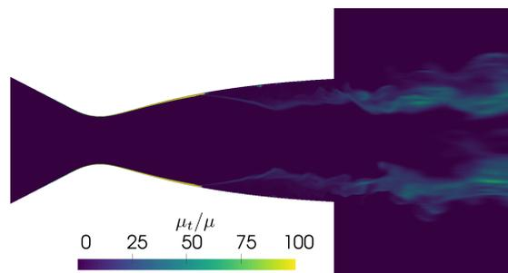
Figure 5.7: Instantaneous DDES solution,  $NPR = 9$ . Contours of turbulent to molecular viscosity ratio ( $\mu_T/\mu$ ). The maximum value of turbulent viscosity is localised at the separation point, with a lower value at the shear layers.
