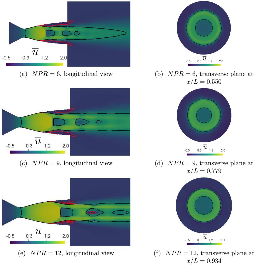
Figure 5.10: Contours of the mean streamwise velocity  $\bar{u}$  at different NPR conditions:  $NPR = 6$  (top),  $NPR = 9$  (middle),  $NPR = 12$  (bottom). The continuous black and red lines are the sonic line and 0-value streamwise velocity isolines, respectively. The transverse slice are taken just downstream the first Mach disk.
