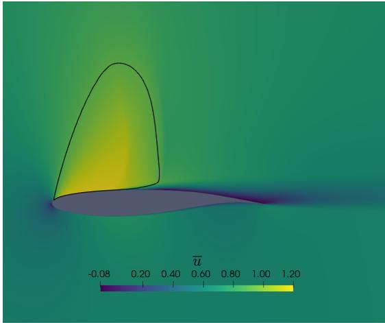
(a) Meanflow streamwise velocity contours. The black line is the sonic line.
