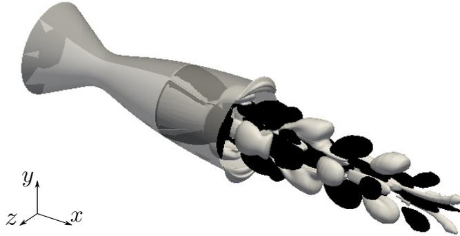
(b) radial velocity mode component  $\hat{u}_r$
