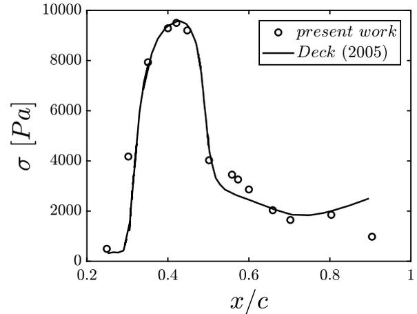
(b) Comparison in terms of pressure RMS ( $\sigma$ ) between current unsteady calculation (empty circles) and an analogous 2D URANS calculation (continuous line) performed by *Deck* (2005) [35] for different streamwise wall locations.  $c$  is the coord length.
