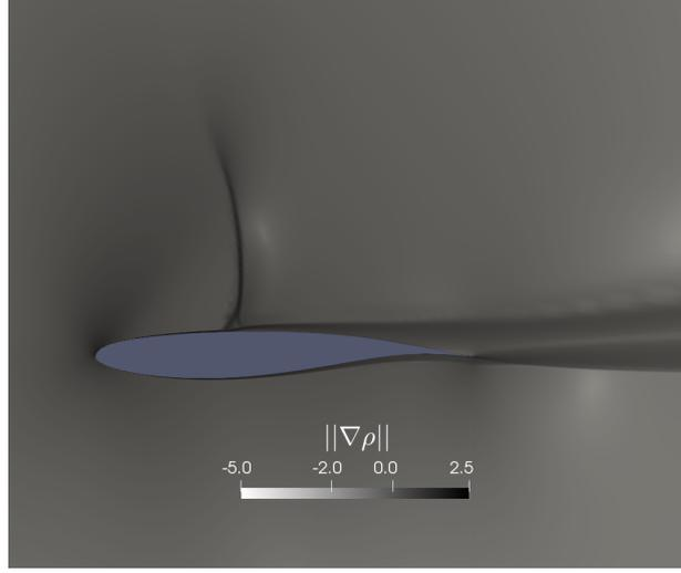
Figure 4.17: Unsteady solution for a 2D transonic turbulent flow past an OAT15A airfoil at  $\alpha_\infty = 4.5^\circ$ : instantaneous density gradient ( $\|\nabla\rho\|$ ) contour in logarithmic scale. A strong lambda shock is well visible on the airfoil surface.
