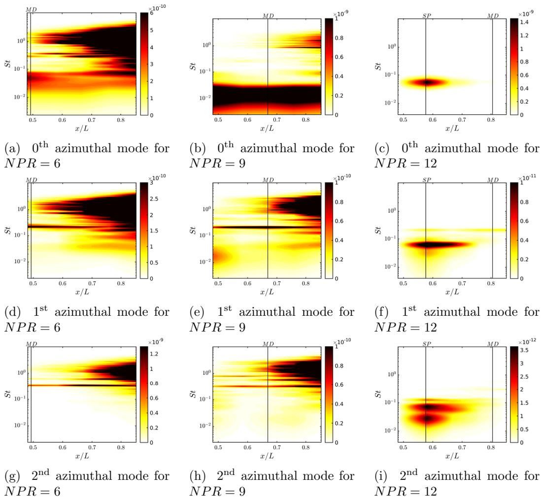
Figure 5.21: Contours of premultiplied PSD for main azimuthal mode of wall pressure perturbation ( $St \langle p_m p_m^* \rangle$ ) in space and frequency domain. The black lines denote the separation point (*SP*) and the location of the first Mach Disk (*MD*), respectively.
