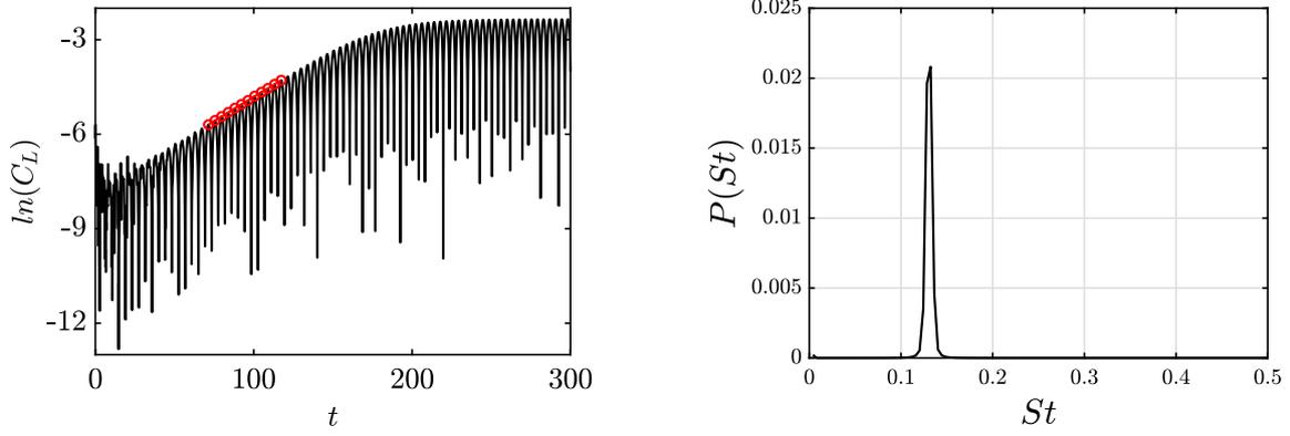
(a) Lift coefficient trend with time, starting from base flow. The red dotted line slope represents the growth-rate ( $\sigma_{NL}$ ).
