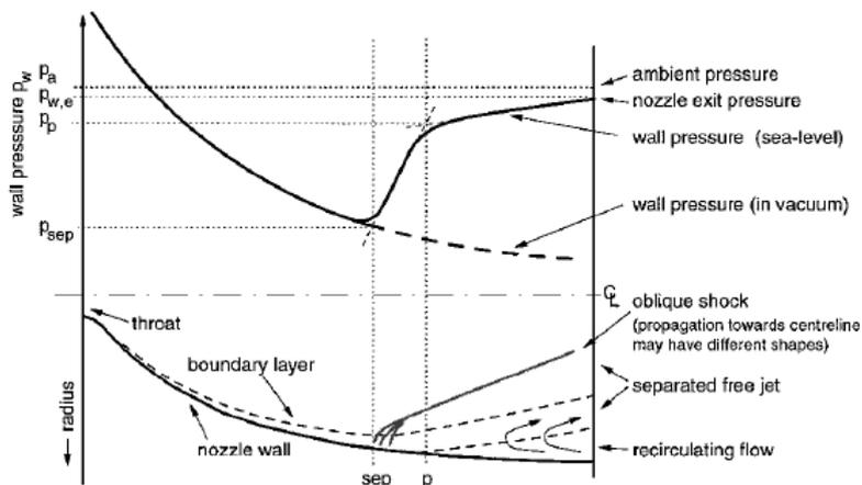
Figure 1.8: Free-shock separation in overexpanded rocket nozzles, wall pressure profile, and phenomenology:—, compression waves/shock, and - - -, boundary/shear-layer edge. From *Frey et al.* (2000) [9]
