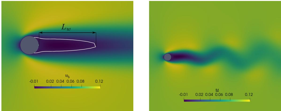
(a) Base flow solution. White lines are isolines at null streamwise velocity and represents the boundary of the wake bubble.  $L_w$  denotes the length wake.
