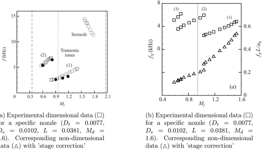
Figure 1.14: Difference between screench and transonic tones, from *Zaman et al.* (2002). The dashed line represents the condition when the flow is just choked ( $p_l$  pressure condition in Figure 1.2), the dotted line when a normal shock is expected at the nozzle exit ( $p_{usu}$  pressure condition in Figure 1.2), and the chain-dashed line when the flow is adapted ( $p_{a,d}$  pressure condition in Figure 1.2).
