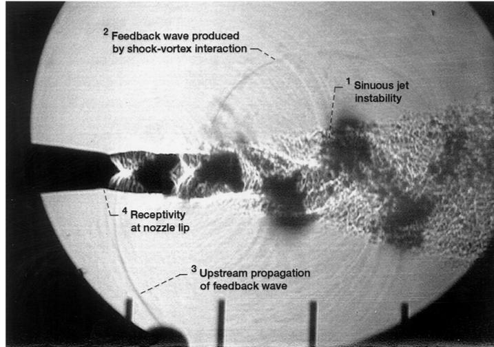
Figure 1.12: Resonant screech loop mechanism, by *Raman* (1998)[11].
