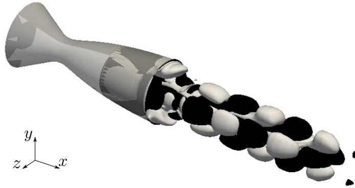
(a) streamwise velocity mode component  $\hat{u}_x$
