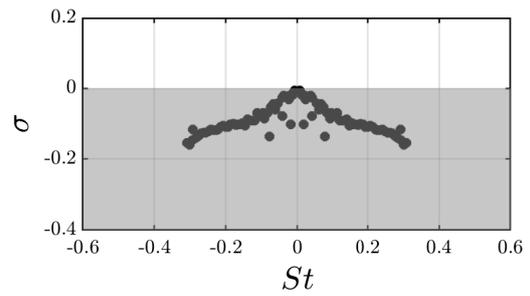
(b) Linear Stability Analysis around meanflow (LURANS). No unstable modes are visible.
