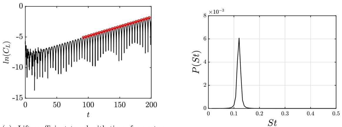
(a) Lift coefficient trend with time, for perturbation. The red dotted line slope represents the perturbation growth-rate ( $\sigma_L$ ).
