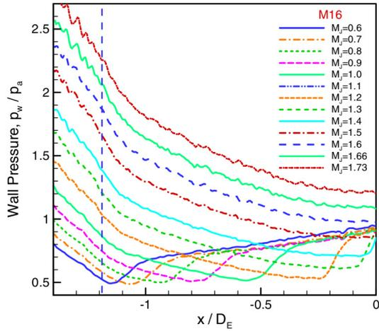
(b) Wall pressure ratio ( $p_w/p_a$ ) trend with  $M_j$  for a  $M_d = 1.6$  convergent-divergent nozzle. From *Zaman et al.* (2015) [22].
