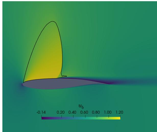
Figure 4.15: Base flow calculation for a 2D transonic turbulent flow past an OAT15A airfoil at  $\alpha_\infty = 4.5^\circ$ : streamwise velocity contours. The solid black line is the sonic line.
