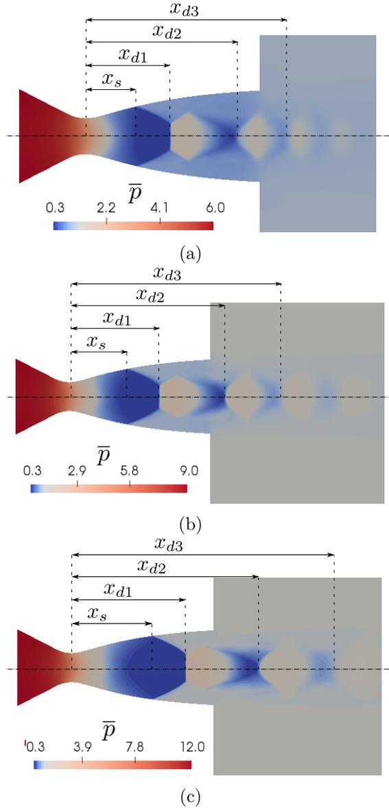
Figure 5.9: Mean DDES solution at different NPR conditions:  $NPR = 6$  (top),  $NPR = 9$  (middle),  $NPR = 12$  (bottom), longitudinal view. Contours of mean pressure  $\bar{p} = \bar{p}^*/p_a^*$ . The colorscale is centered at  $\bar{p} = \bar{p}^*/p_a^* = 1$  (i.e. where mean pressure  $\bar{p}$  matches ambient pressure  $p_a$ ) to highlight the shock system.
