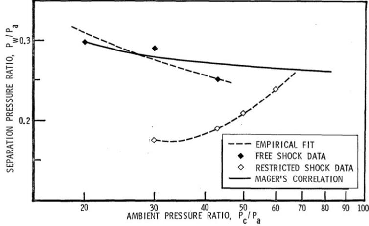
(a) Separation pressure ratio ( $p_w^{\min}/p_a = NPR \cdot p_w^{\min}/p_0$ ) trend with NPR ( $p_c/p_a = p_0/p_a$ ) for FSS and RSS regimes. From *Nave & Coffey* (1973) [21]
