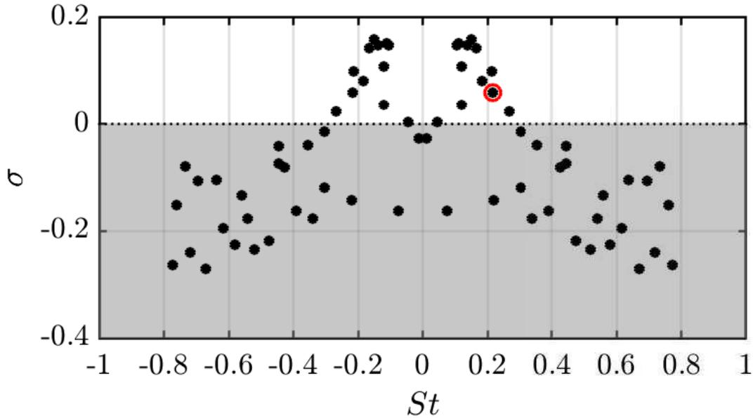
Figure 5.26: Nozzle Flow at  $NPR = 9$ . Eigenspectrum for Global Stability Analysis around the mean flow. An unstable mode  $(\sigma, St) = (0.06, 0.22)$  matching the unsteadiness at  $St^{NL} \approx 0.2$  is denoted with an empty red circle. Conversely, another mode at  $St = 0.3$ , which can be probably associated to the nonlinear activity with symmetry  $m = 2$ , is stable.
