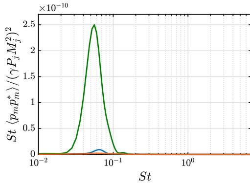
(e) DDES calculation for  $NPR = 12$  at  $x/L = 0.665$
