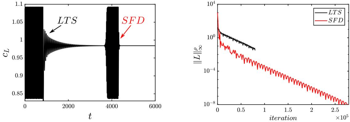
(a) Lift coefficient trend under *flow-unleash* method. Firstly, LTS method is activated on the saturated limit cycle in order to get an approximated steady solution. Secondly, instabilities are left to naturally develop and limit cycle is reached again. Finally, SFD is properly activated to stabilise the unsteady solution.
