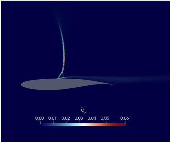
(b) Real part of streamwise velocity component mode  $\hat{u}_x$  for global unstable mode at  $(\sigma, St) = (0.054, 0.055)$
