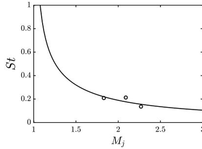
Figure 5.20: Comparison between *Tam's* correlation (1986) [12] and 1<sup>st</sup> azimuthal mode peak frequency at different values of NPR ( $M_j$ )
