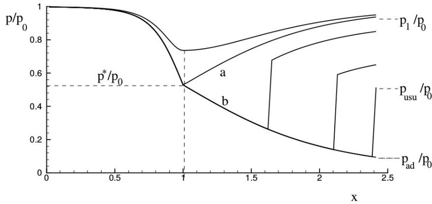
Figure 1.2: Nozzle flow at different  $\text{NPR} = p_0/p$  for a fully operational engine ( $p_0 = p_{0,d}$ ): adapted flow for  $\text{NPR} = p_0/p_{a,d}$ ; sonic flow throat pressure  $p^*$ ; oblique shock at exit for  $\text{NPR} = p_0/p_{usu}$ ; supersonic-subsonic flow with inner or outer shock occurrence for  $p_0/p_1 < \text{NPR} < p_0/p_{usu}$ ; pure subsonic flow with  $\text{NPR} < p_0/p_1$ .  $p_1$  and  $p_{a,d}$  are called limit pressure and adaptation pressure, respectively.
