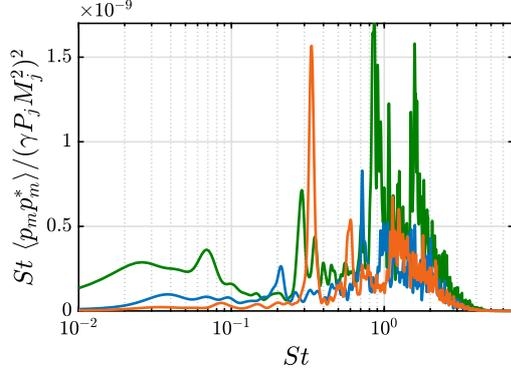
(a) DDES calculation for  $NPR = 6$  at  $x/L = 0.665$
