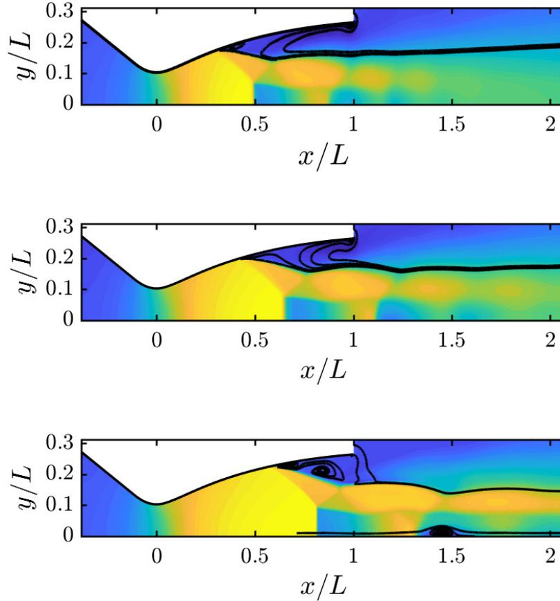
Figure 5.11: Contours of the mean streamwise velocity  $\bar{u}$  at different NPR conditions:  $NPR = 6$  (top),  $NPR = 9$  (middle),  $NPR = 12$  (bottom). Streamlines are denoted with a solid black line. Two recirculation regions are well visible near the nozzle lip and the separation shock. In addition, for the nozzle flow at  $NPR = 12$ , a trapped vortex is visible downstream the second Mach disk.
