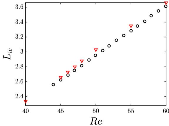
Figure 4.4: Base flow calculation: length of the bubble wake ( $L_w$ ) for different Reynolds number ( $Re$ ). Red triangles correspond to the current simulation, black empty circles to data from *Giannetti & Luchini* (2007) [1].
