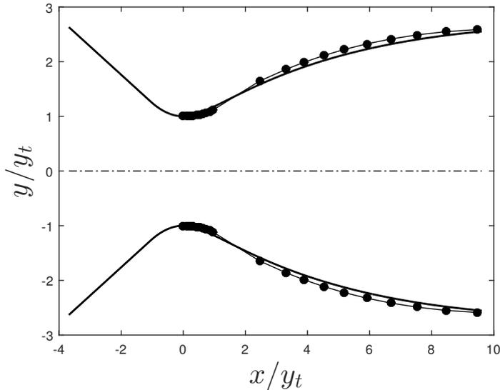
Figure 5.3: Nozzle Contour. TIC nozzle geometry (continuous line), Ideal Contour nozzle obtained by MOC (filled circles line), symmetry axis (dashed line).  $y_t$  corresponds to the throat radius  $R_t$ .
