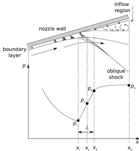
Figure 1.5: Phenomenology of shock separation. At the incipient separation point, wall pressure increases sharply from  $p_i$  to a plateau pressure  $p_p$ . After that, pressure slightly increases until exit up to  $p_e$ . From *Aghababaie & Theunissen* (2015) [6]
