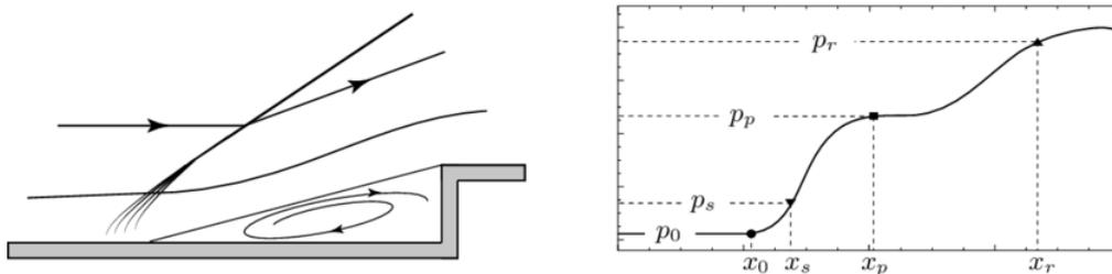
Figure 1.7: Supersonic flow over forward-facing steps from *Matheis & Hickel* (2015)[8]. A restricted ricirculation region is visible bewteen separation point and the forward facing step (left). Near separation, wall pressure rapidly increases from  $p_s$  to a plateau value  $p_p$  and then more slowly once more up to  $p_r$  where flow reattaches (right).
