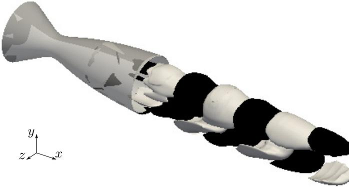
(c) azimuthal velocity mode component  $\hat{u}_\theta$
