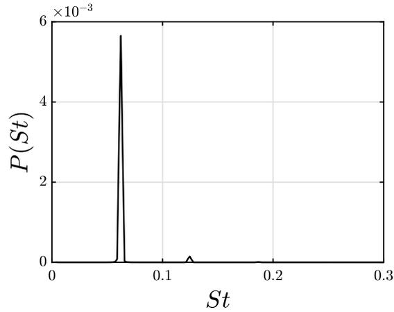
Figure 4.19: Unsteady solution for a 2D transonic turbulent flow past an OAT15A airfoil at  $\alpha_\infty = 4.0^\circ$ : a peak at  $St_{NL} = 0.0623$  is well visible with no too much energetic harmonics.
