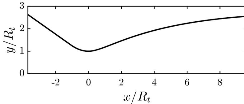
Figure 5.1: TIC nozzle axisymmetric geometry,  $M_d = 3.5$ .
