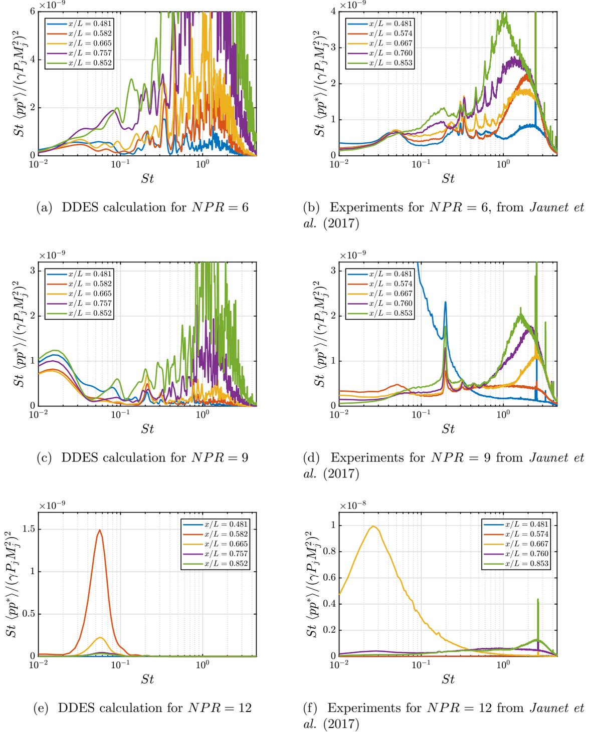
Figure 5.18: Premultiplied PSD of wall pressure perturbation for different streamwise locations at azimuth position  $\theta = 180^\circ$ .
