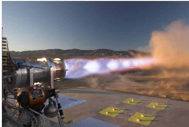
Figure 1: Shock diamonds structure during 5M15 engine firing up test in Mojave Desert. From Wired [3]
