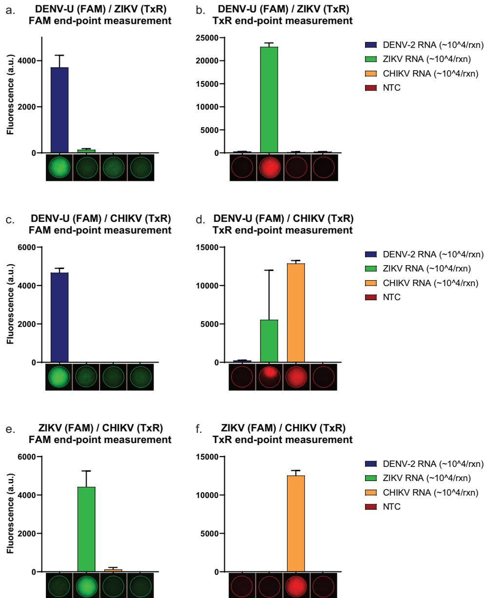
**FIGURE 3.13** – rt-LAMP des trois duplexes QUASR (a) DENV-U(FAM)/ZIKV(Texas Red), Canal FAM (b)DENV-U(FAM)/ZIKV(Texas Red), Canal Texas Red (c) DENV-U(FAM)/CHIKV(Texas Red), Canal FAM (d)DENV-U(FAM)/CHIKV(Texas Red), Canal Texas Red (e) ZIKV(FAM)/CHIKV(Texas Red), Canal FAM (f)ZIKV(FAM)/CHIKV(Texas Red), Canal Texas Red
