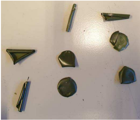
Figure II- 27 Flatness maintenance during thermal treatment. A) Sintering without weight; B) Sintering with weight
