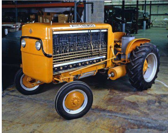
Figure 2 Allis Chalmers fuel cell tractor (source image: Smithsonian institute [24])
