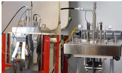
Figure IV - 4 Electrochemical measurements set-up. A) Fiaxell testing rig; B) Brook Instruments debit flow meter (figure II-38C)
