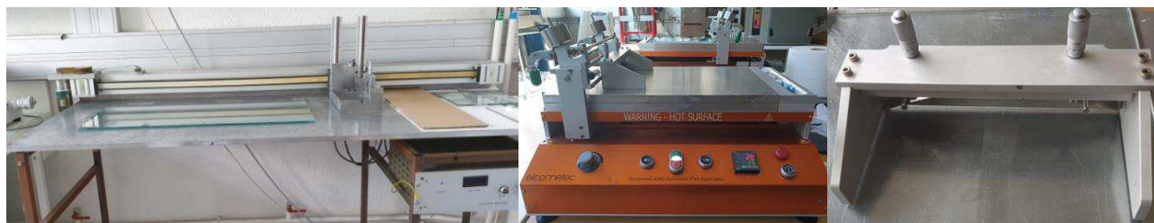
Figure II-18 Tape casting equipment. A) Homemade tape casting bench; B) Commercial Elcometer 4340 tape caster; C) Elcometer 3580 doctor blade;
