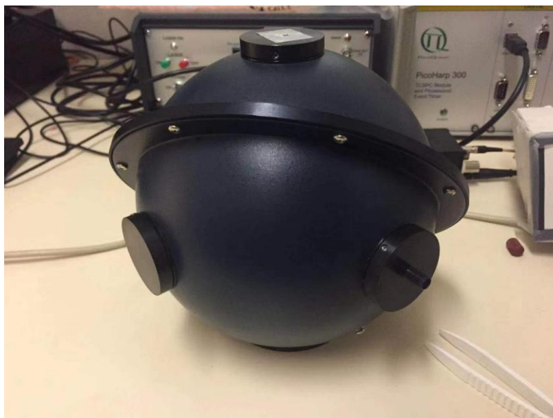
Figure 2.1 The integrating sphere that was used in the measurement of internal UCQY.
