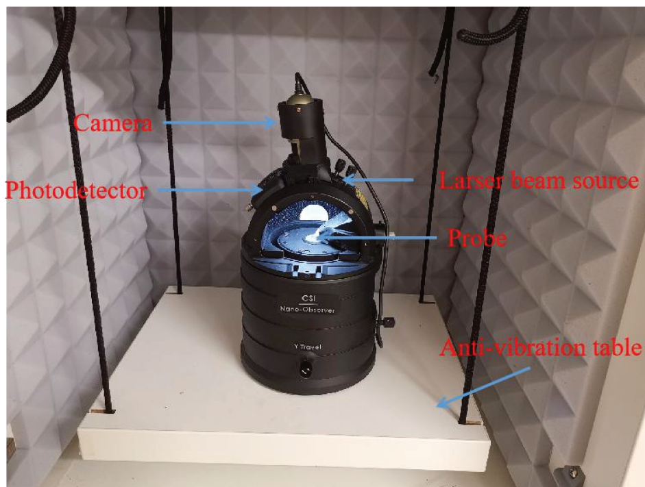
Figure II-11 Nano-Observer AFM microscope used in this work
