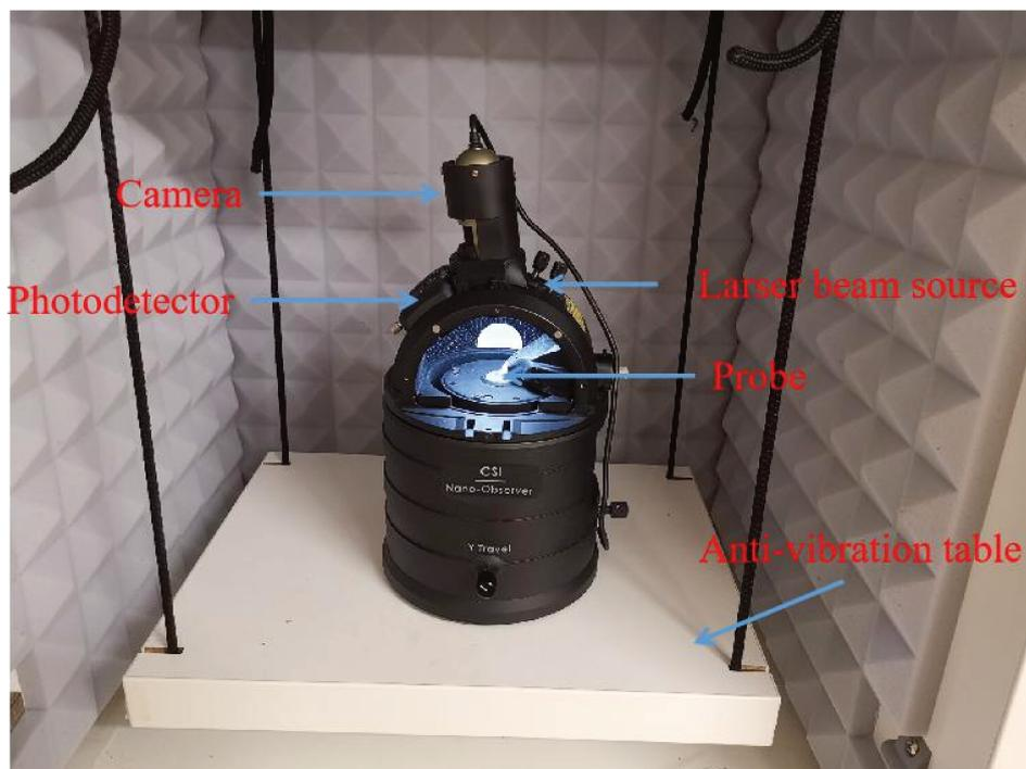
Figure II-11 Nano-Observer AFM microscope used in this work
