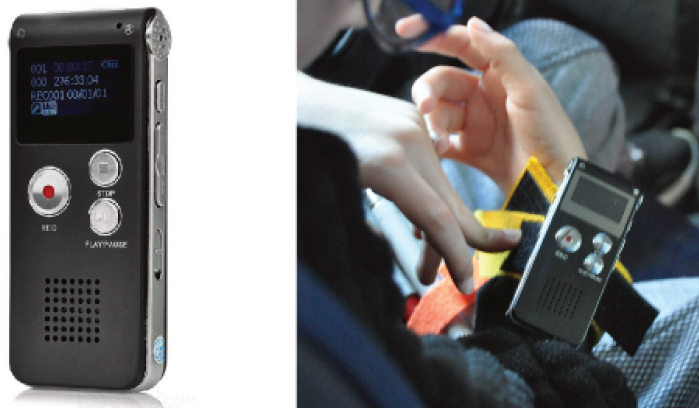
Figure 14.2: The second version of the probe is worn on the wrist. It consists of a strap covered with velcro on which an audio recorder/player. It has three main buttons that are tactilely recognizable, one to start recording, the second to stop recording and the third to play the last recording.
