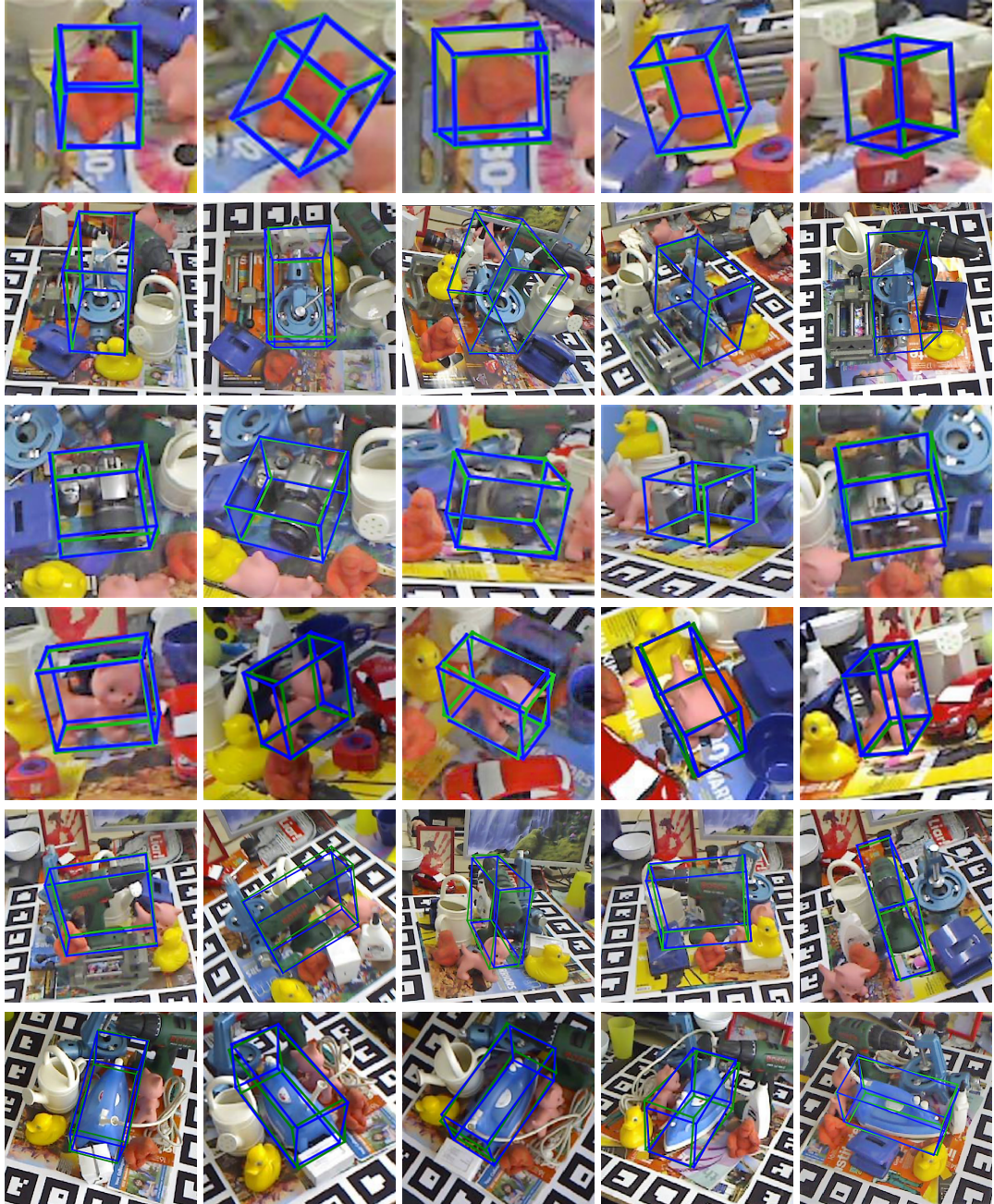
Figure 3.8: Qualitative results of our pose estimation method on LINEMOD [46]. green : ground-truth 3D bounding box; blue : 3D bounding box estimated by our method.
