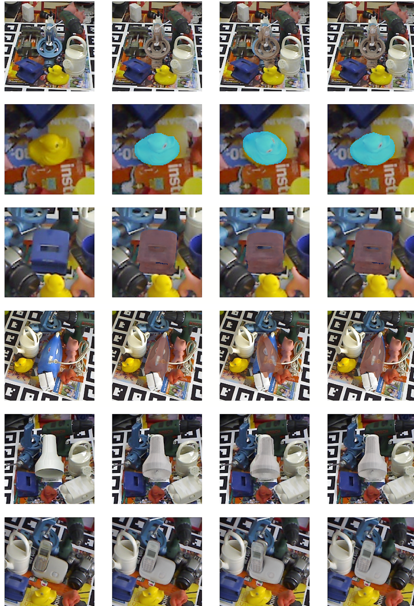
Figure 3.10: Qualitative results of our pose refinement method on LINEMOD [46]. For each sample, the four columns from left to right represent: the input image, the rendered object with the ground-truth pose, the rendered object with the initial pose estimate by our initial pose estimator [152] and the rendered object with refined pose.
