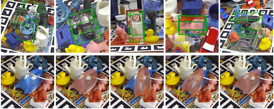
Figure 1.2: Examples of the object 6D pose estimation task and the pose refinement task. The first row presents some objects whose poses are to be estimated where the green bounding boxes are the projected object 3D bounding boxes using the ground-truth 6D poses; The second row presents the iterative pose refinement of an object, from left to right: the input image, the rendered object using the ground-truth pose, the rendered object using the initial pose estimate, the rendered object using the first pose update, the rendered object using the second pose update.
