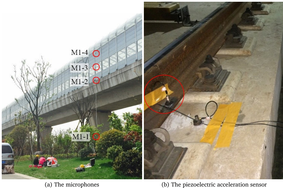
Fig 3.2.: Part of the apparatus used on the site with a barrier during the measurement
