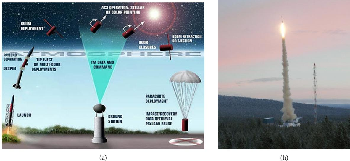
Figure 2.10: (a) A parabolic flight profile [21]. (b) Successful launch of TEXUS-42 sounding rocket [22].
