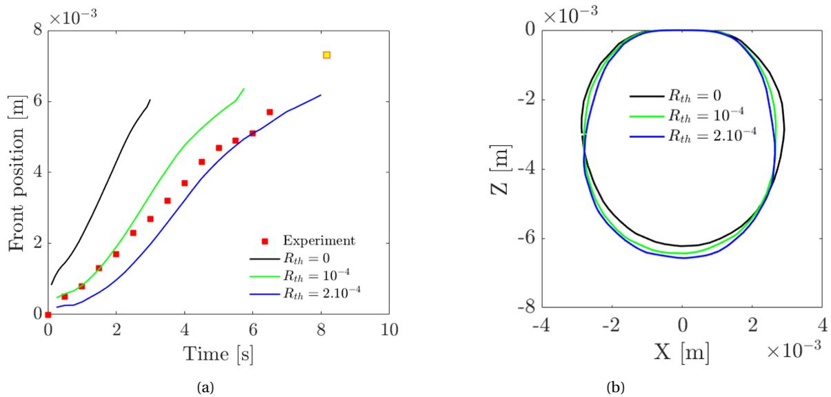
Figure 5.15: Comparison of 2D simulations with  $R_{th}=0 \text{ W}^{-1} \cdot \text{m}^2 \cdot \text{K}$ ,  $R_{th} = 10^{-4} \text{ W}^{-1} \cdot \text{m}^2 \cdot \text{K}$  and  $R_{th} = 2 \cdot 10^{-4} \text{ W}^{-1} \cdot \text{m}^2 \cdot \text{K}$  for (a) time evolution of the solidification front position and (b) the final droplet shapes
