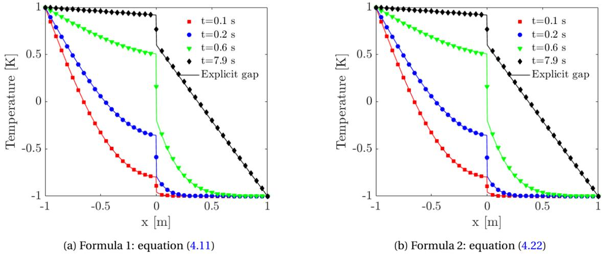
Figure 4.13: Time-evolution of the temperature jump across the interface for  $C_{p,G} = \mathcal{O}(\overline{C}_p)$
