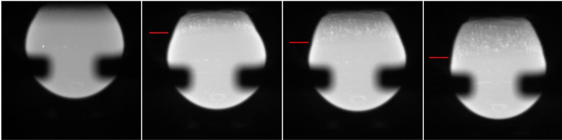
Figure 2.7: Sequence of video images for the Fe-0.1C-0.2Si experiment showing the sample shape time evolution (from left to right). The time increment between images is 0.5 s starting at the time of contact with the chill plate at 25.9 s. The chill plate (not visible) was located at the top and moved downwards. The red line marks the position of the growth front. From the video taken at 500 fps growth velocity is determined to approximately  $1\text{mm}\cdot\text{s}^{-1}$  [20].
