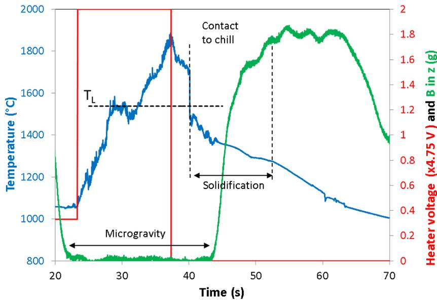
Figure 2.8: Time evolutions for a Fe-0.05C-0.2Si sample during a chill cooling cycle in TEMPUS parabolic flight: (blue) temperature, (red) heater control voltage and (green) microgravity level.
