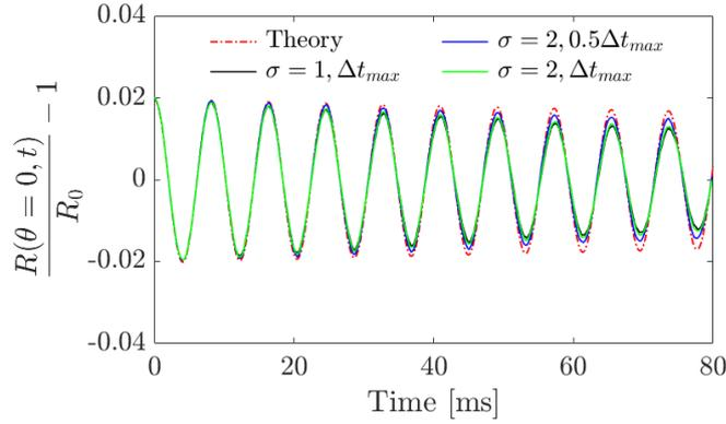
Figure 3.12: Comparison of the oscillation radius simulated with the 1<sup>st</sup> order of discretisation of Navier-Stokes and the radius simulated with 2<sup>nd</sup> order with different time steps
