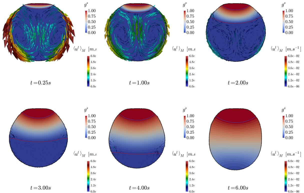
Figure 5.16: Snapshots of the solidifying droplet showing temperature field superimposed to the velocity of the metal at different times. The red and blue lines mark the position of  $g^s = 1\%$  and  $g^s = 99\%$  respectively
