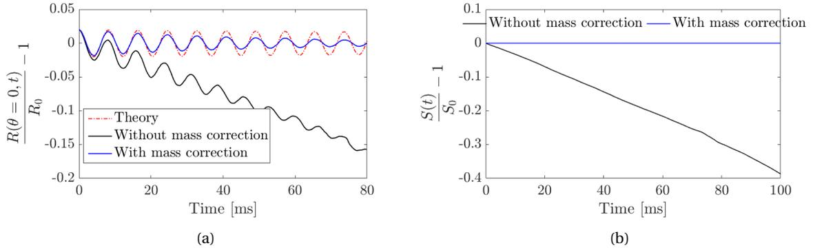
Figure 3.7: (a) Comparison of the time-evolutions of the radius of the drop without mass correction (black line), the radius with mass correction (blue line) and the theoretical solution (red line)
