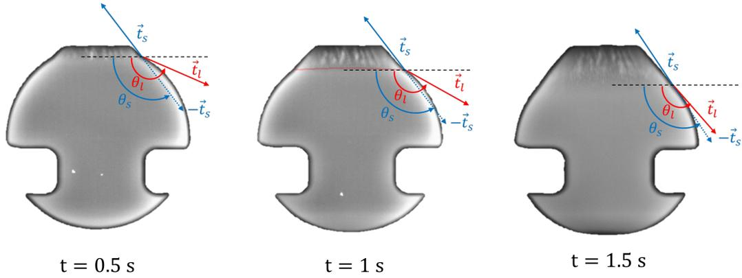
Figure 2.20: Snapshots showing differences in solid and liquid angles at the solidification front position. The liquid angle  $\theta_l$  is marked in red and the solid angle  $\theta_s$  is marked in blue.
