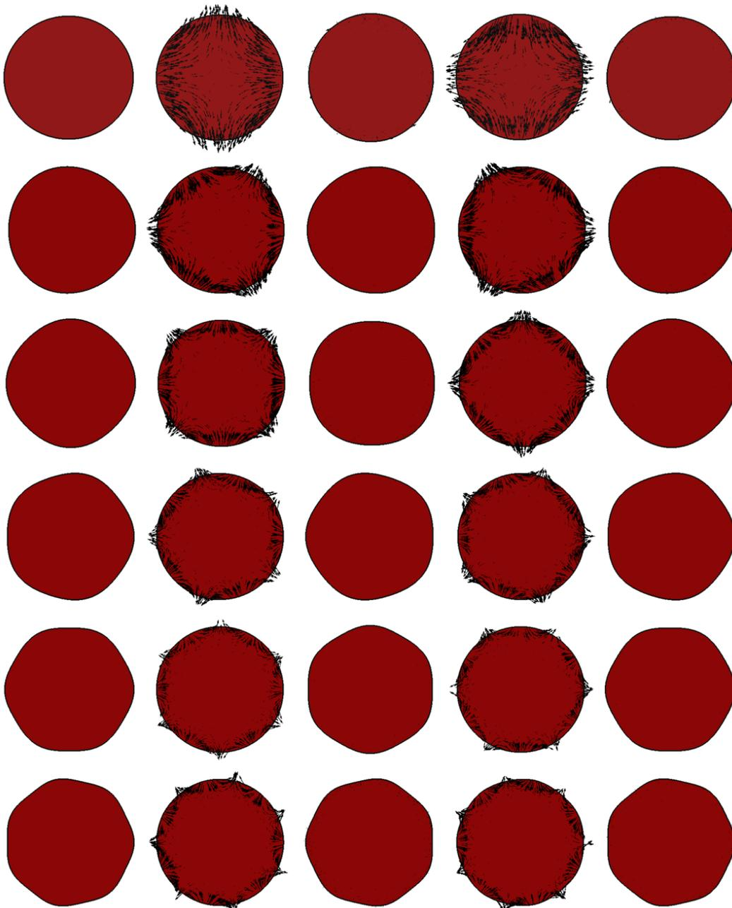
Figure 3.14: The time-evolution of the droplet shape over the first oscillation period for modes from  $n = 2$  (upper row) to  $n = 7$  (lower row). From the left column to the right, time corresponds to  $t=0, \frac{T_n}{4}, \frac{T_n}{2}, \frac{3T_n}{4}$  and  $T_n$  respectively
