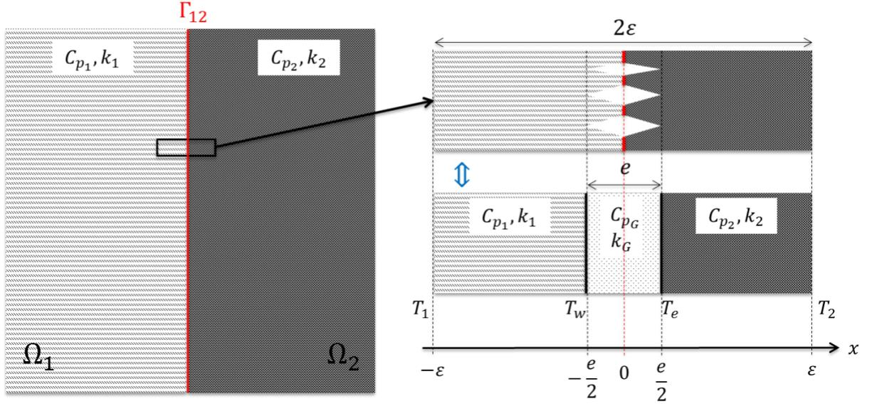
Figure 4.2: Schematic of two materials in contact,  $\Omega_1$  and  $\Omega_2$ , forming a thermally resistant interface  $\Gamma_{12}$  due to the presence of a gap layer,  $\Omega_G$ , with thickness  $e$ .
