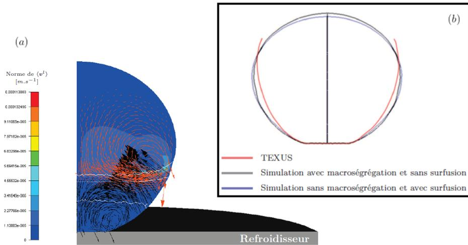
Figure 1.4: (a) Numerical simulation showing the velocity field of the solid phase (black arrows) and the liquid phase (orange arrows) at  $t = 1.5$  s during the solidification of a 3.3mm radius steel droplet. (b) Droplet shape predicted by numerical simulation with macrosegregation (grey) and without macrosegregation (blue) in comparison with TEXUS experimental profile (red) at  $t = 4.5$  s [12]. The top of the experimental shape was not visible in the experiment.
