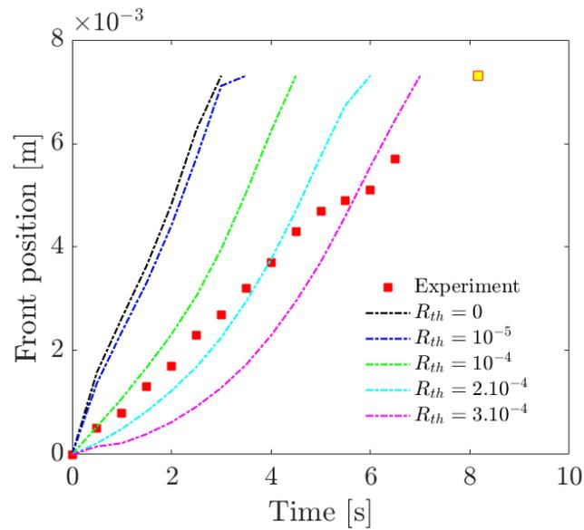
Figure 5.14: Parametric study in 2D pure conduction in which the thermal contact resistance is varying from 0 to  $3 \cdot 10^{-4} \text{ W}^{-1} \cdot \text{m}^2 \cdot \text{K}$ . The numerical results are plotted in dashed lines. The measured front position is marked by red squares. The yellow square is the final front position extrapolated form measurements.
