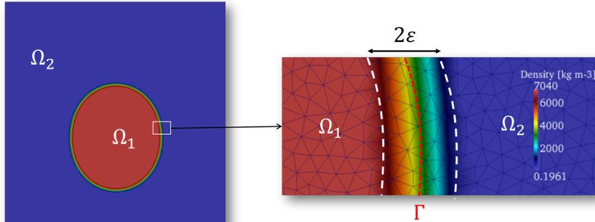
Figure 3.2: The diffuse interface approach illustrated via the density profile across the interface
