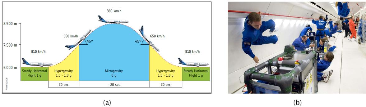
Figure 2.2: (a) A parabolic flight profile [18]. (b) View inside the Zero-G Airbus aircraft during the 46<sup>th</sup> ESA flight campaign [19].
