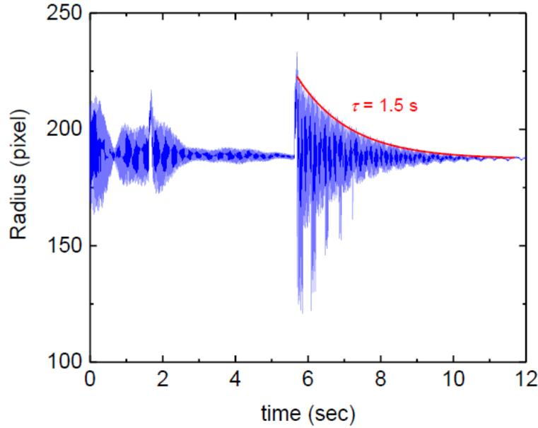
Figure 2.23: The time evolution of the oscillation of the radius of the droplet [25].
