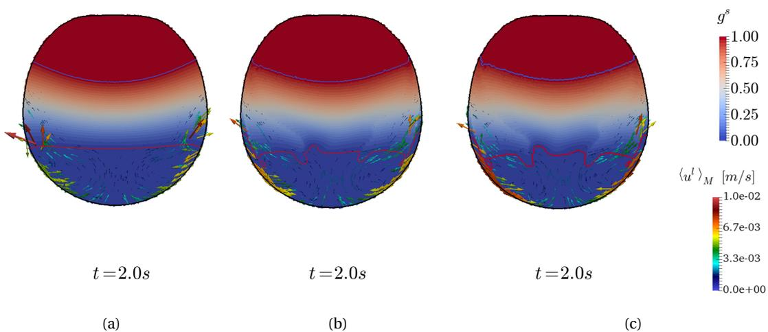
Figure 5.9: Comparison of the solid fraction field at the time  $t = 2s$  for (a) a binary alloy with a constant and uniform Carbon composition, (b) a binary alloy with Carbon transport and (c) a ternary alloy with Carbon and Silicon transport. The red and blue lines mark the position of the iso-values  $g^s = 1\%$  and  $g^s = 99\%$  respectively
