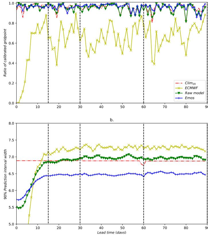
Figure 3.6: a. Ratio of calibrated gridpoints over the domain as a function of the forecast lead time. Knuppel test is performed at significance level  $\alpha = 0.01$  on the S-PIT built from 48 forecasts. b. 90% prediction interval width averaged over the domain and all forecast sets as a function of the forecast lead time.
