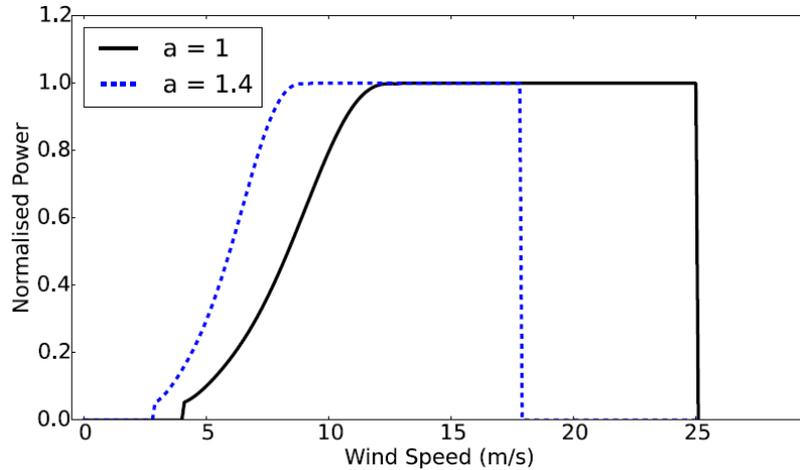
Figure 2.7: *Power curve*: Example of the location-adapted power curve. In solid black: the real power curve for wind speed at 80m height; in dashed blue: the adapted power curve. It has the same shape, but the wind speed is divided by a number  $a$  to achieve a capacity factor of 23%.
