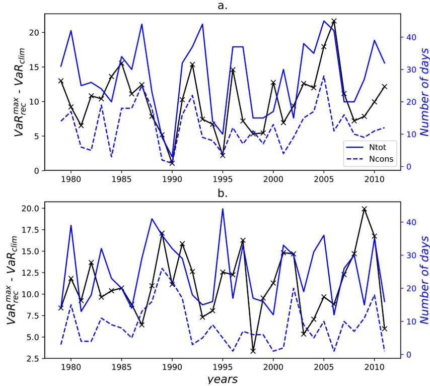
Figure 4.8: Difference between the maximum  $VaR_{95}$  and the climatological  $VaR_{95}$  (86GW) (black line), total number of days (blue line) and maximum number of consecutive days (dashed blue line) when the predicted  $VaR_{95}$  is superior to the climatological  $VaR_{95}$  for winter (a.) and fall (b.) seasons
