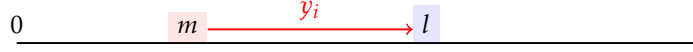
Figure 3.1: 1D toy SLAM problem. A robot at position m observes a landmark at position l with a range measurement y_i .
